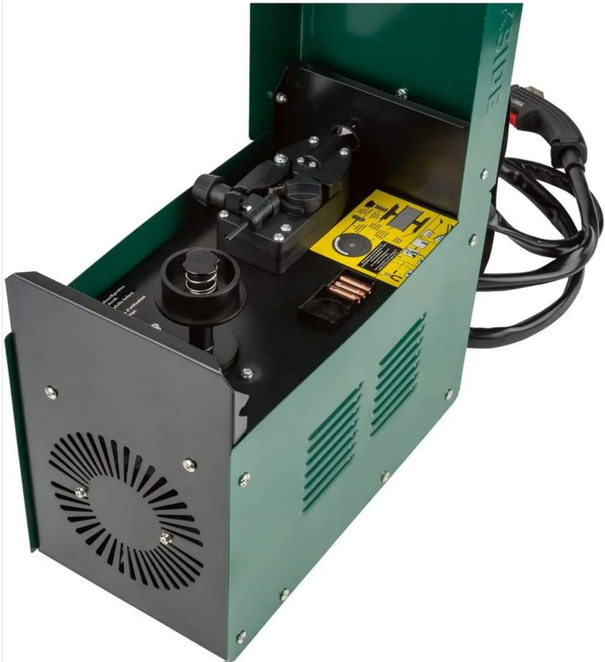
Figure 2.4: Internal view of the welding machine, showing the wire feeder mechanism for the flux-cored wire.
