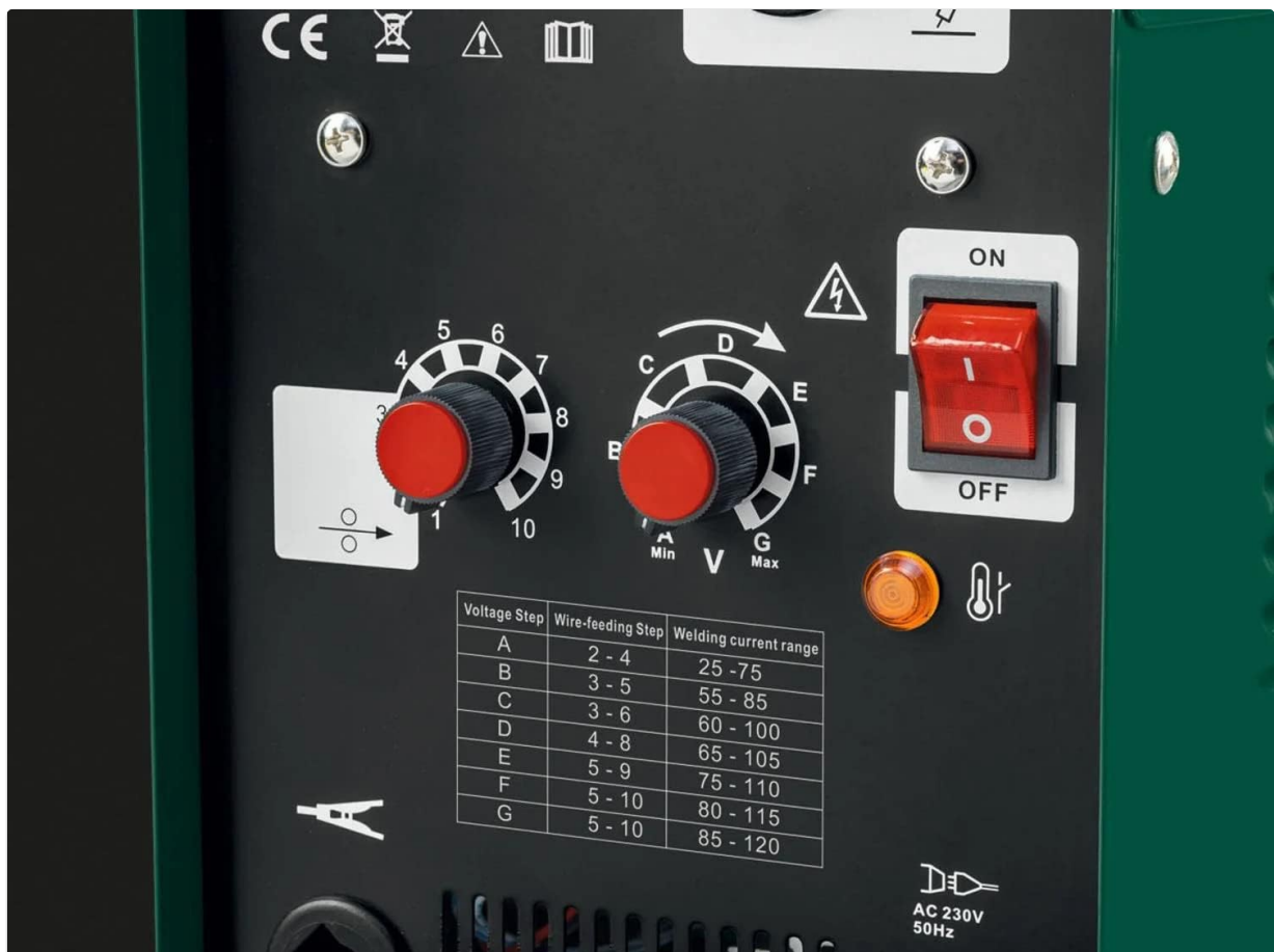
Figure 2.3: Detailed view of the control panel, showing the ON/OFF switch, current adjustment knobs, and the welding parameter table.
