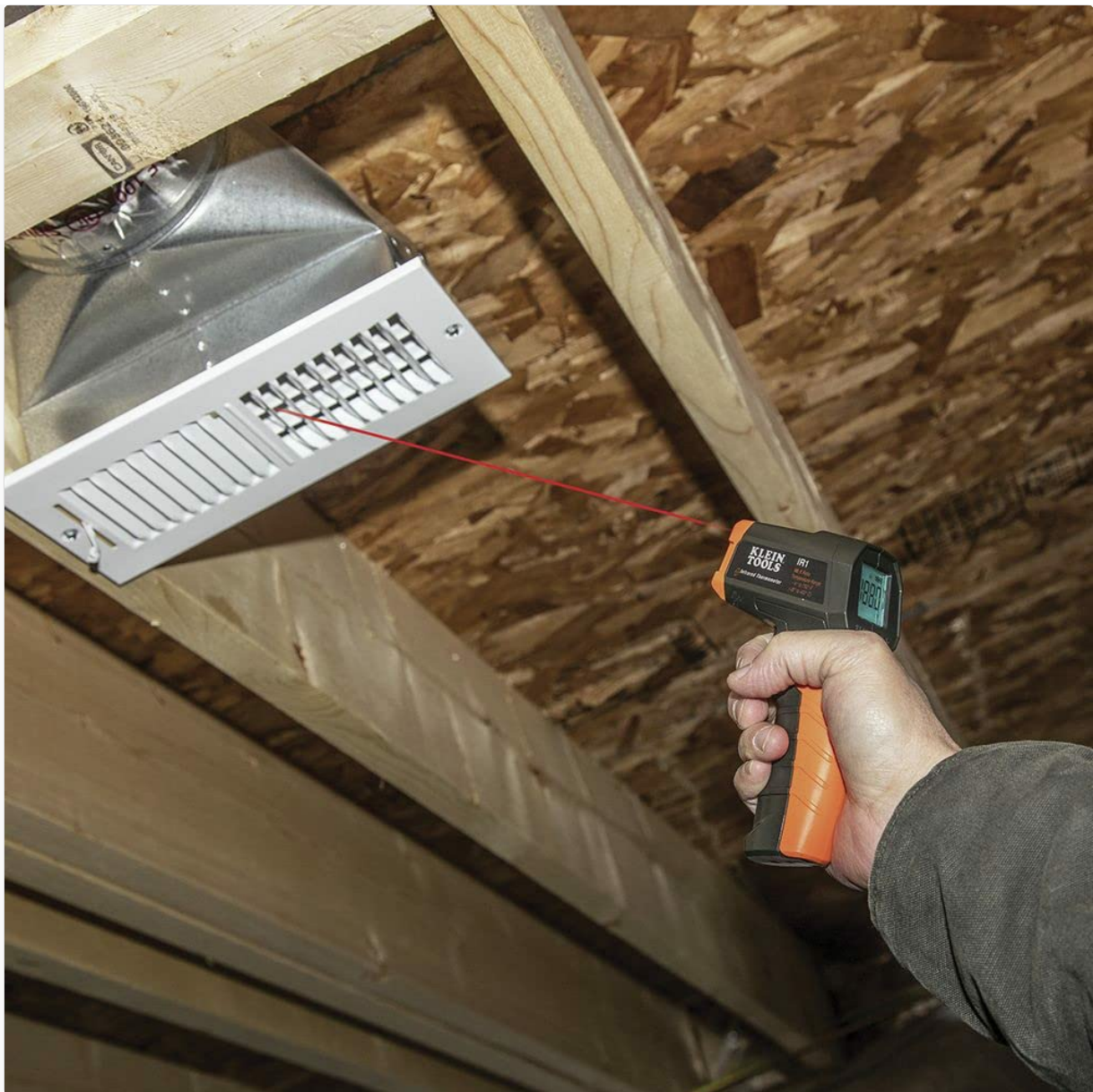
Image: The IR1 thermometer being used to measure the temperature of an HVAC vent, demonstrating its application in environmental diagnostics.
