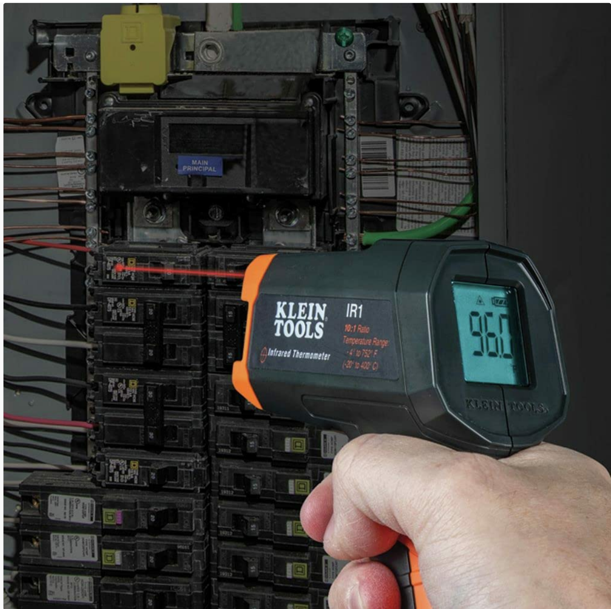
Image: The IR1 thermometer in use, measuring the temperature of components within an electrical panel, with the laser targeting a specific point.
