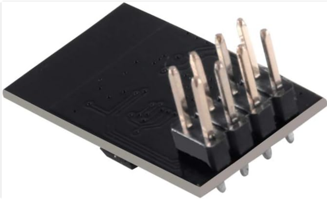
Figure 3: Bottom view of the ESP-01 module showing the pin arrangement.
