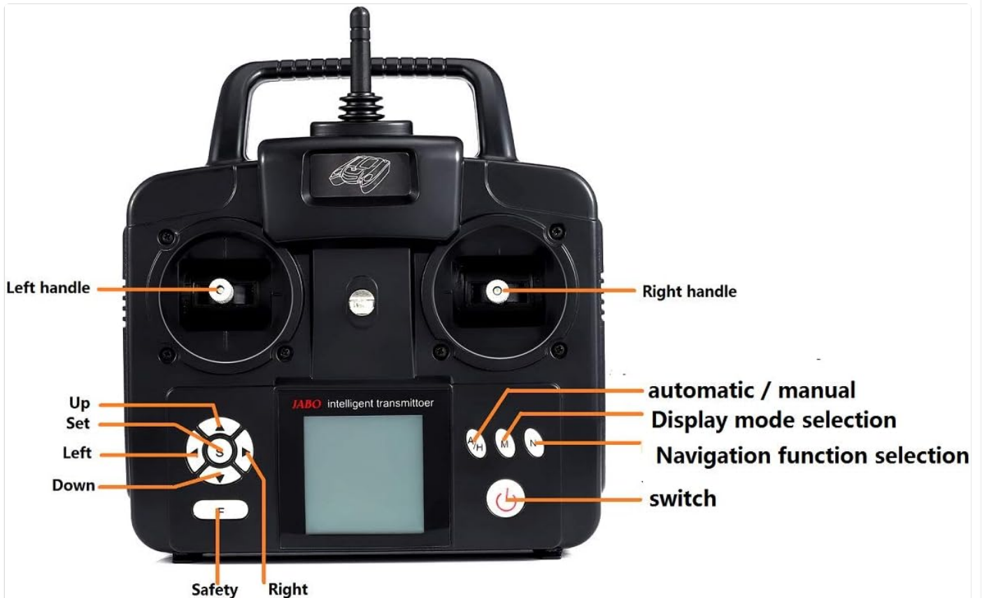
Figure 2.2: Labeled diagram of the JABO 5CG Remote Control, showing the left handle (joystick), right handle (joystick), Up/Set/Left/Down/Right buttons, Safety button, automatic/manual switch, Display mode selection, Navigation function selection, and power switch.
