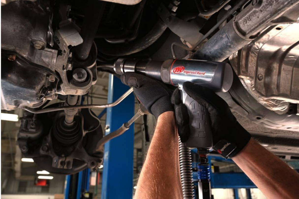
Image: A person wearing gloves operates the Ingersoll Rand 119MAX Air Hammer on an automotive component, demonstrating its use in a workshop setting.
