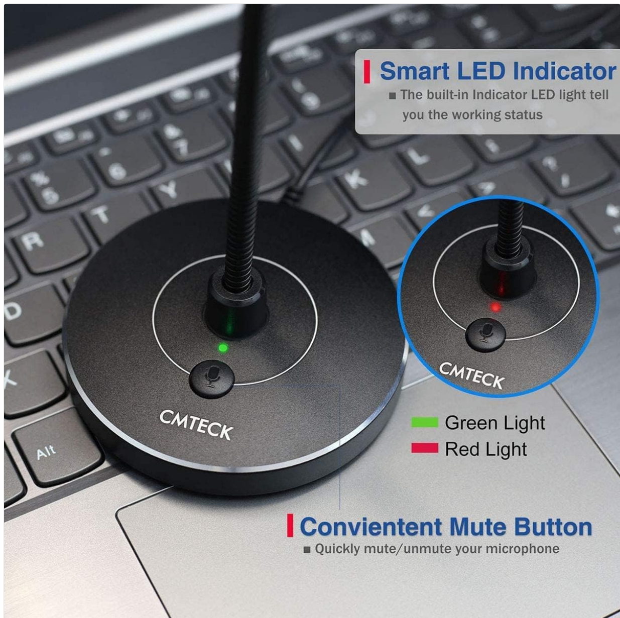
Image: A close-up view of the CMTECK G009 microphone's base, clearly showing the mute button and the LED indicator in both green (connected) and red (mute) states.
