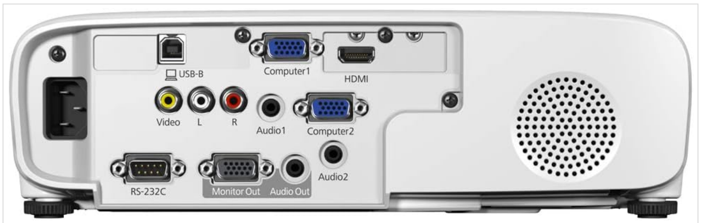
Figure 4: Rear view of the projector showing various input and output ports, including HDMI, USB-B, Computer 1 (VGA), Computer 2 (VGA), Video (RCA), Audio 1 (RCA), Audio 2 (3.5mm), Monitor Out, Audio Out, and RS-232C.
