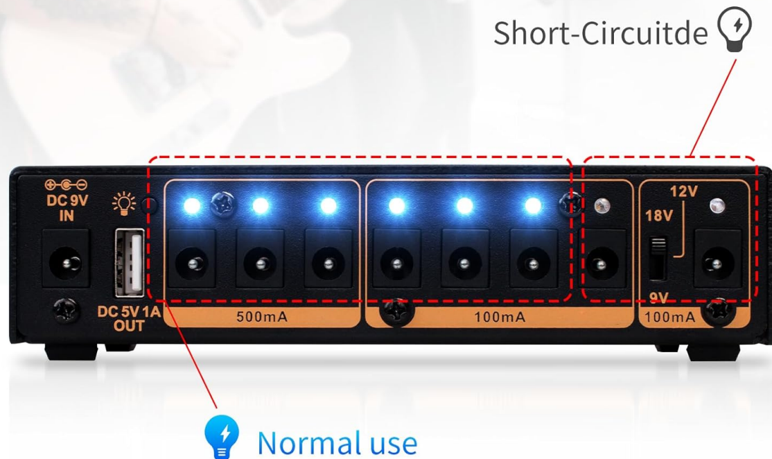
Image 8.1: Illustration of the independent short-circuit protection feature, where a fault in one output does not affect others.
