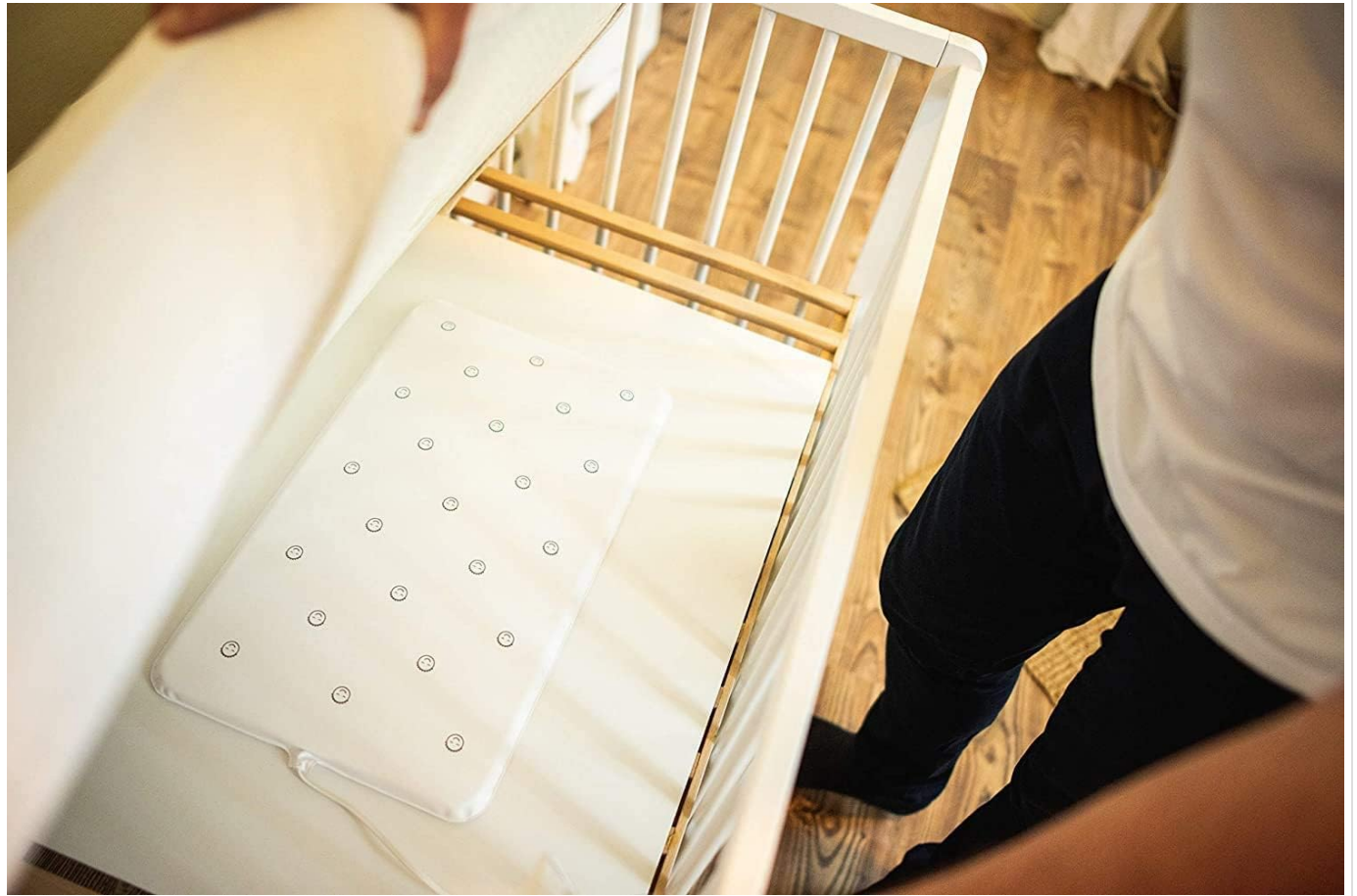
Figure 4.1: Correct placement of the sensor pad under the mattress.
