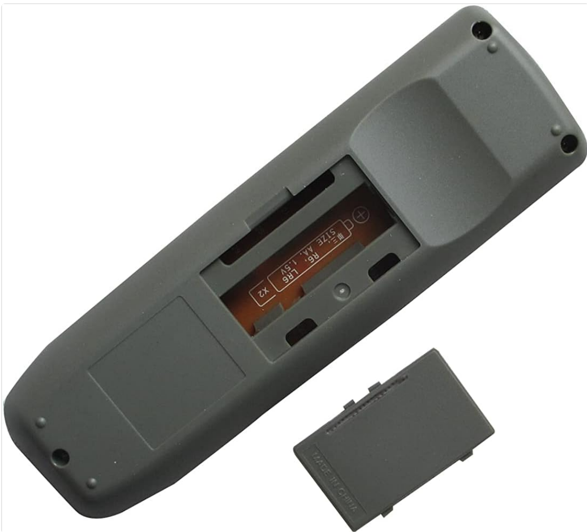
Figure 2: Back view of the remote control with the battery compartment open. This image shows the empty battery slots and the required AA battery size and polarity markings.
