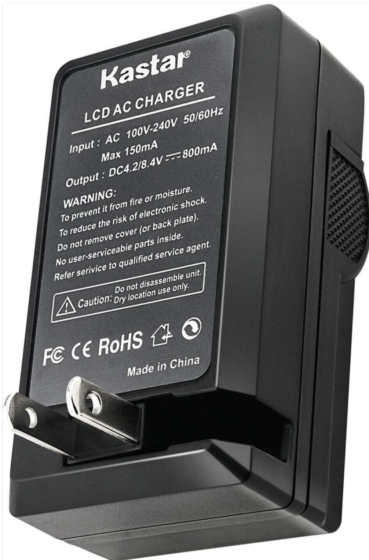
Image: Back of the charger displaying safety warnings and electrical specifications.
