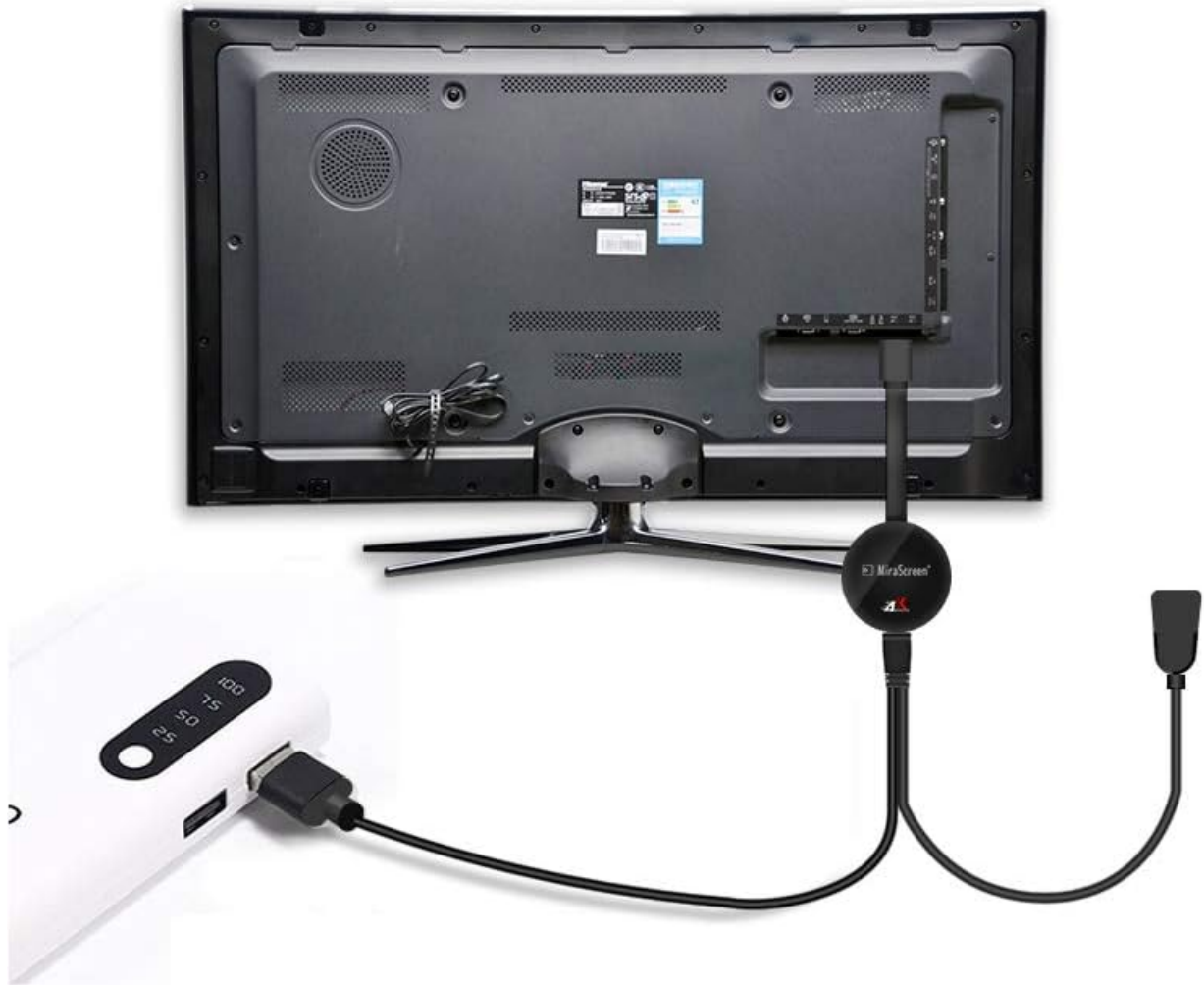
Image: A diagram illustrating the connection of the MiraScreen G7 Plus dongle to a TV, showing the HDMI connection and USB power input from a charger or TV USB port.
