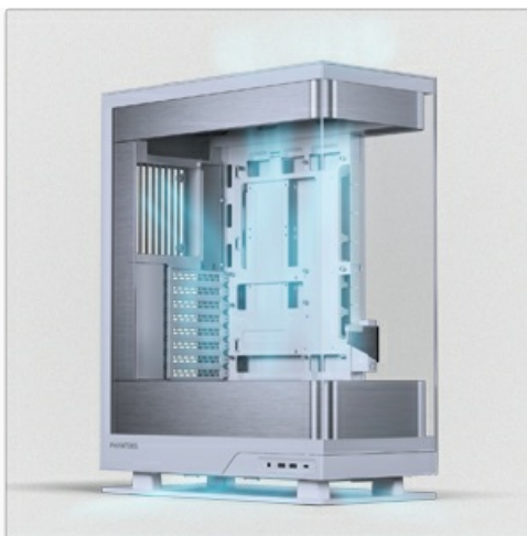
Image: Diagram illustrating the vertical airflow path within the Phanteks Evolv X2 chassis, with air entering from the bottom and exiting from the top.
