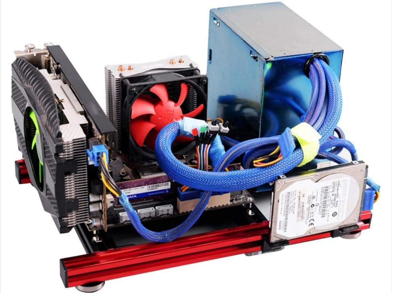
Figure 5: A fully populated test bench demonstrating component placement and cable management.
