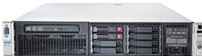
Figure 3.1: Front View of HP ProLiant DL380P G8 Server. This image displays the front panel of the server, showing the 8-bay 2.5-inch drive cages, optical drive, and front panel controls/indicators.
