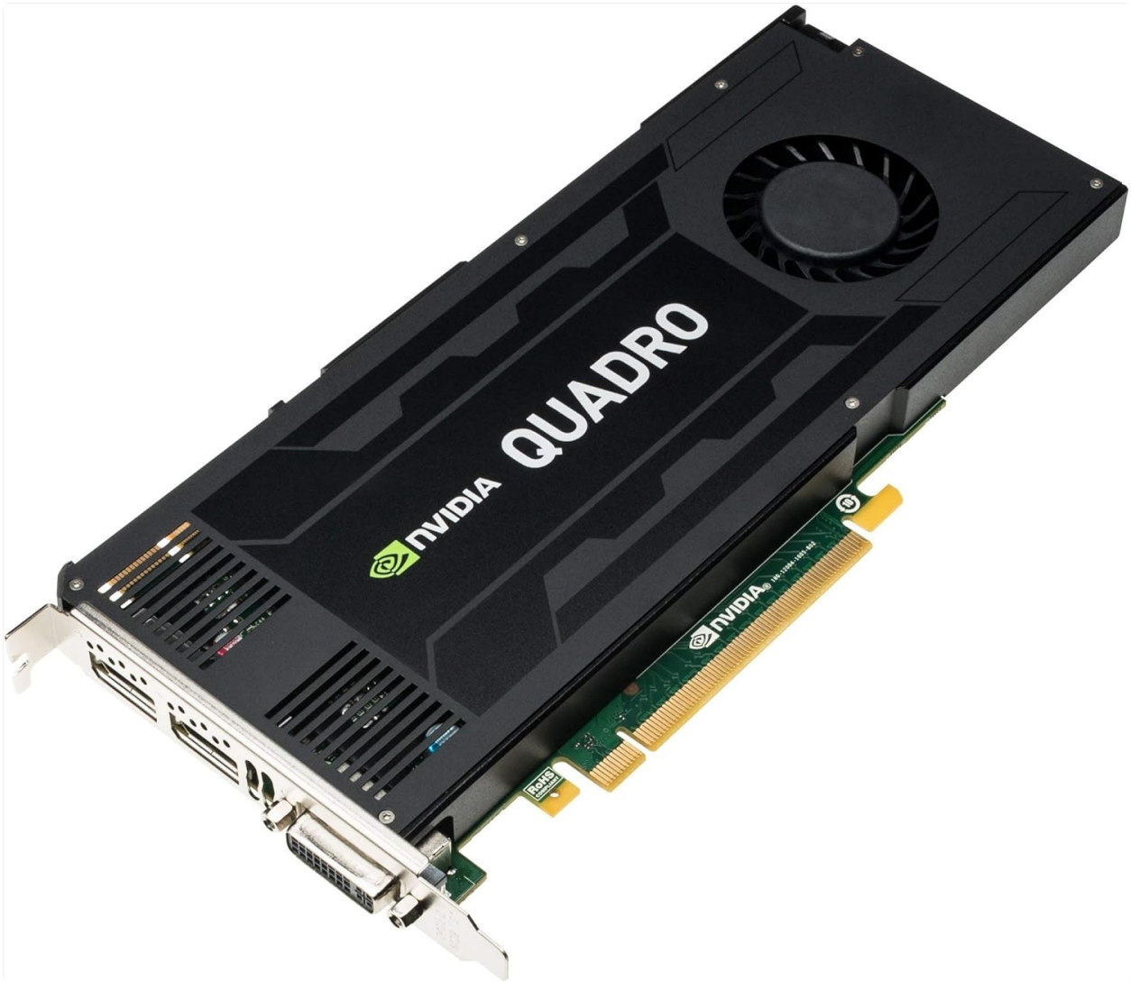
Figure 1: NVIDIA Quadro K4200 Graphics Card. This image displays the full graphics card, highlighting its cooling fan, heatsink, and various output ports including DisplayPort and DVI.
