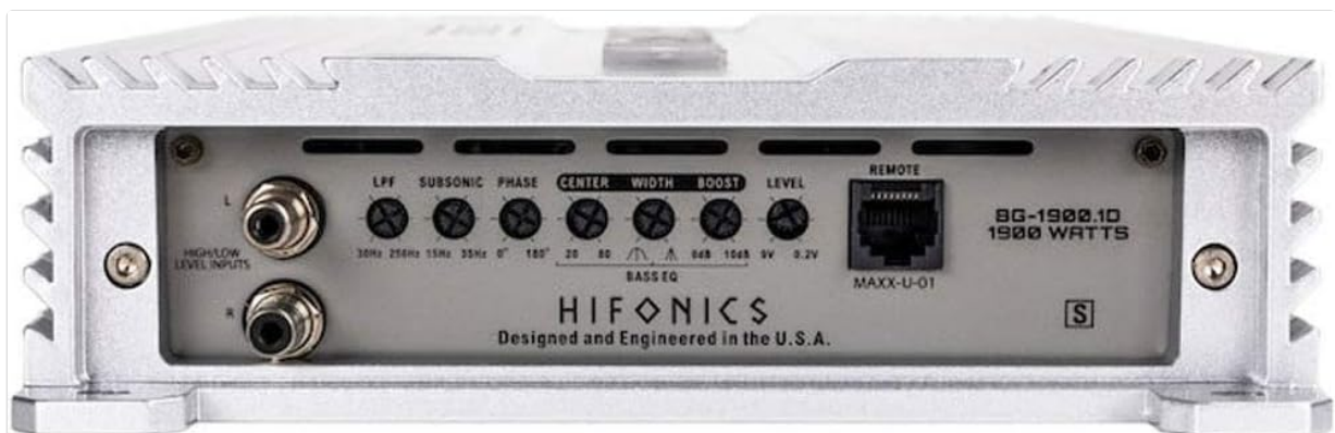
Figure 4.2: Rear panel of the amplifier, detailing the RCA inputs, crossover controls, bass EQ, and level adjustments.
