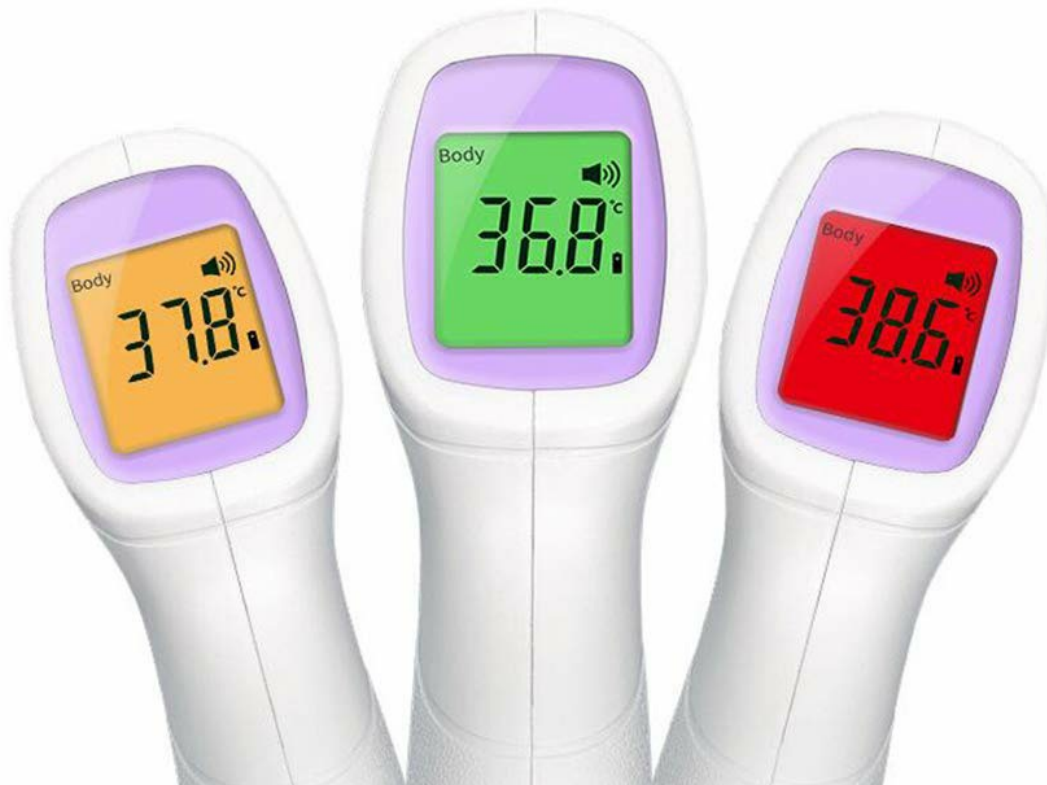
Image 7.1: Visual representation of the three-color backlight system indicating normal, slight fever, and high fever temperature ranges.
