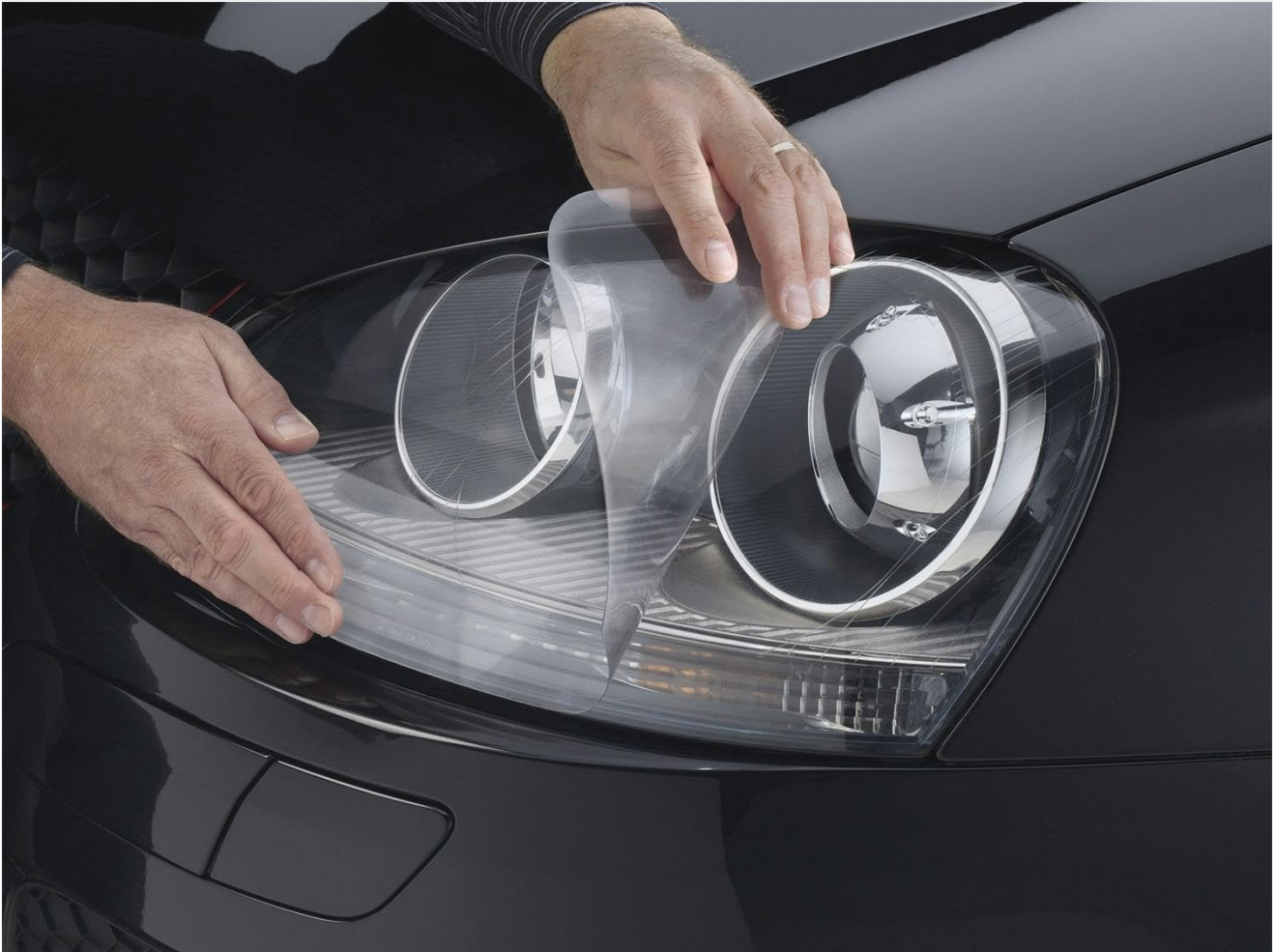
Image: A person's hands carefully applying the clear protective film to a vehicle's headlight.
