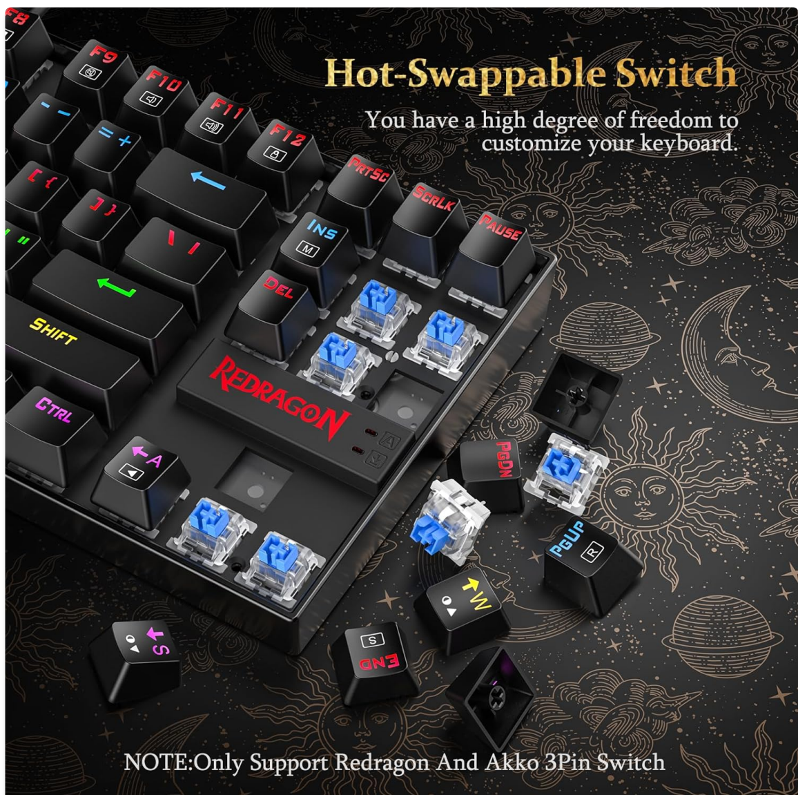
Figure 2: Hot-swappable switch mechanism.
