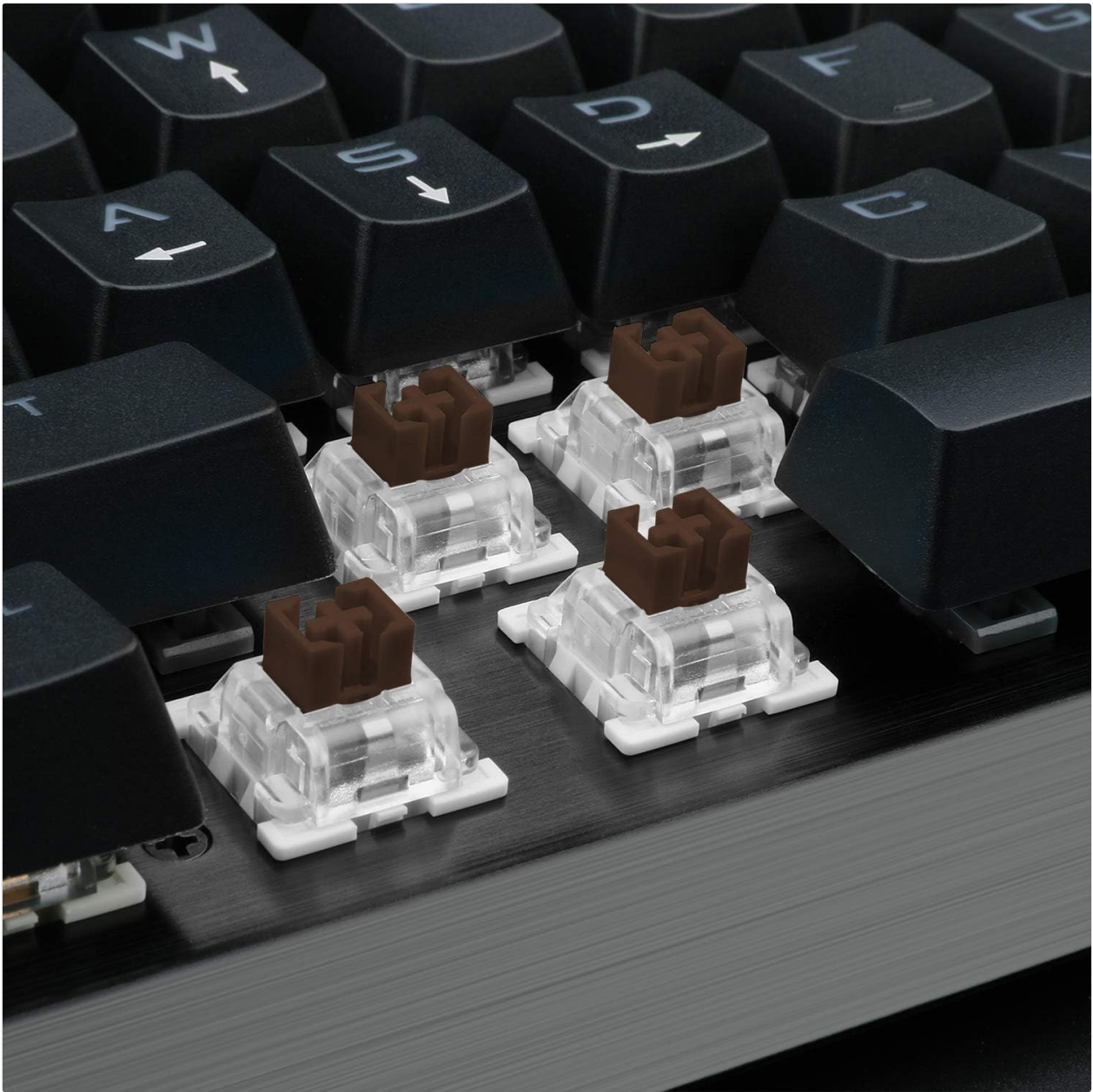
Figure 6.2: Detailed close-up of the brown mechanical switches used in the Eagletec KG010 keyboard, showing their construction.
