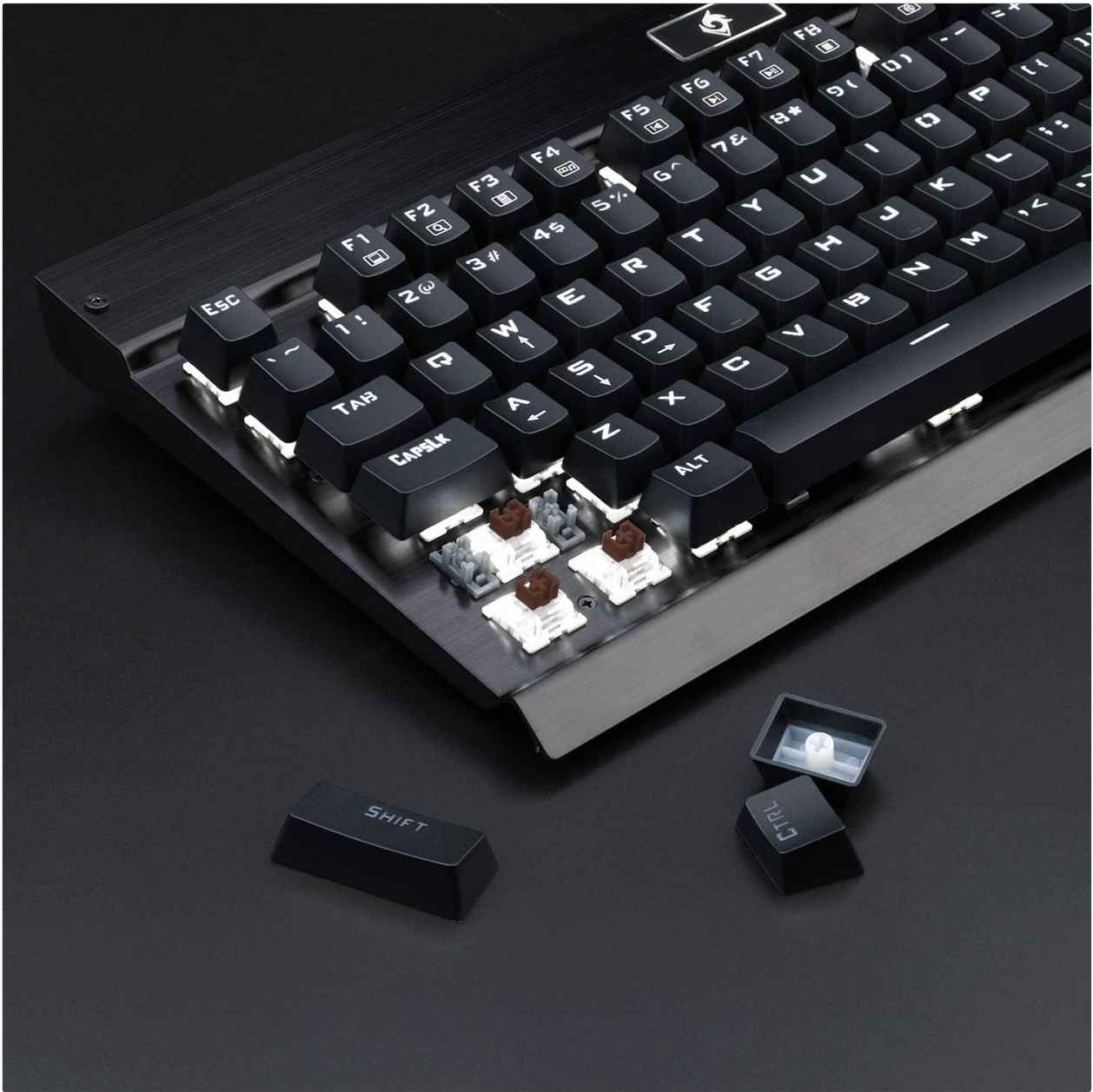
Figure 6.1: Close-up view of the Eagletec KG010 Mechanical Keyboard with several keycaps removed, revealing the brown mechanical switches and the white LED backlighting.
