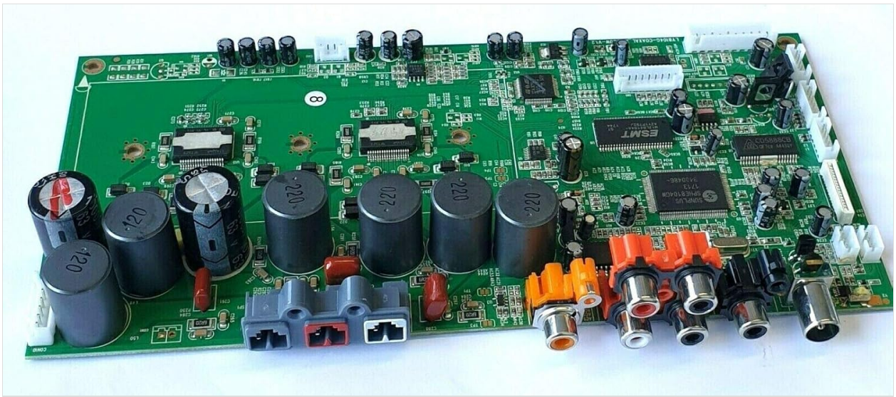
Figure 1: Top view of the Tibo LY8104G Coaxal_IN-750W V1.2 Main Board. This image displays the primary components, including capacitors, integrated circuits, and various input/output connectors such as RCA jacks and power terminals. The board is green with multiple surface-mounted components.
