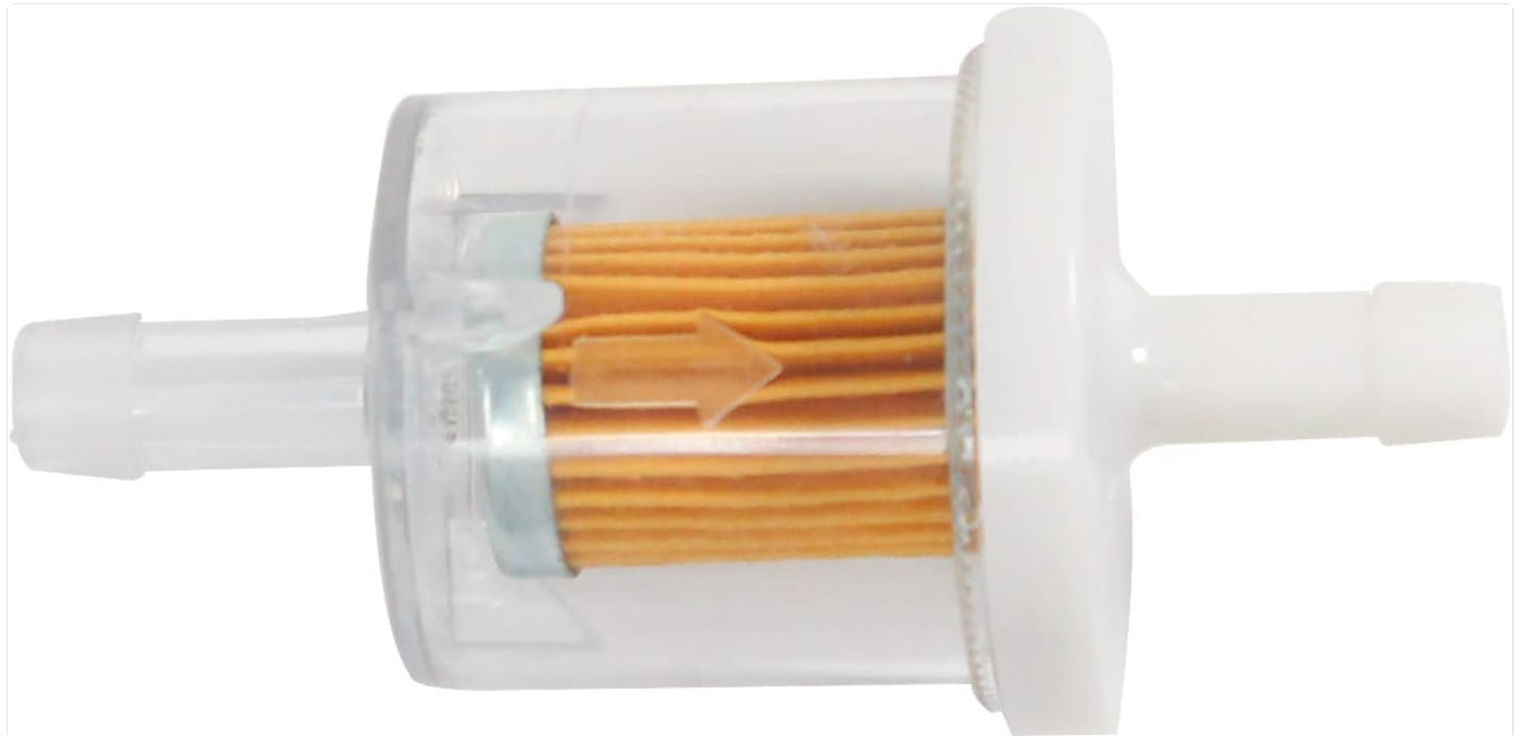
Figure 3.2: Side view of the fuel filter, highlighting the direction of fuel flow indicated by an arrow on the filter body. Ensure this arrow points towards the engine during installation.
