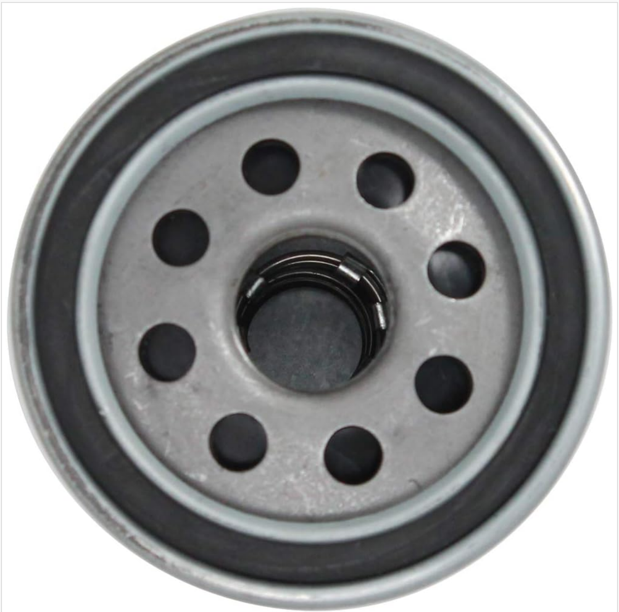
Figure 1: Top view of the oil filter, highlighting the gasket and oil passages. Apply oil to the rubber gasket before installation.
