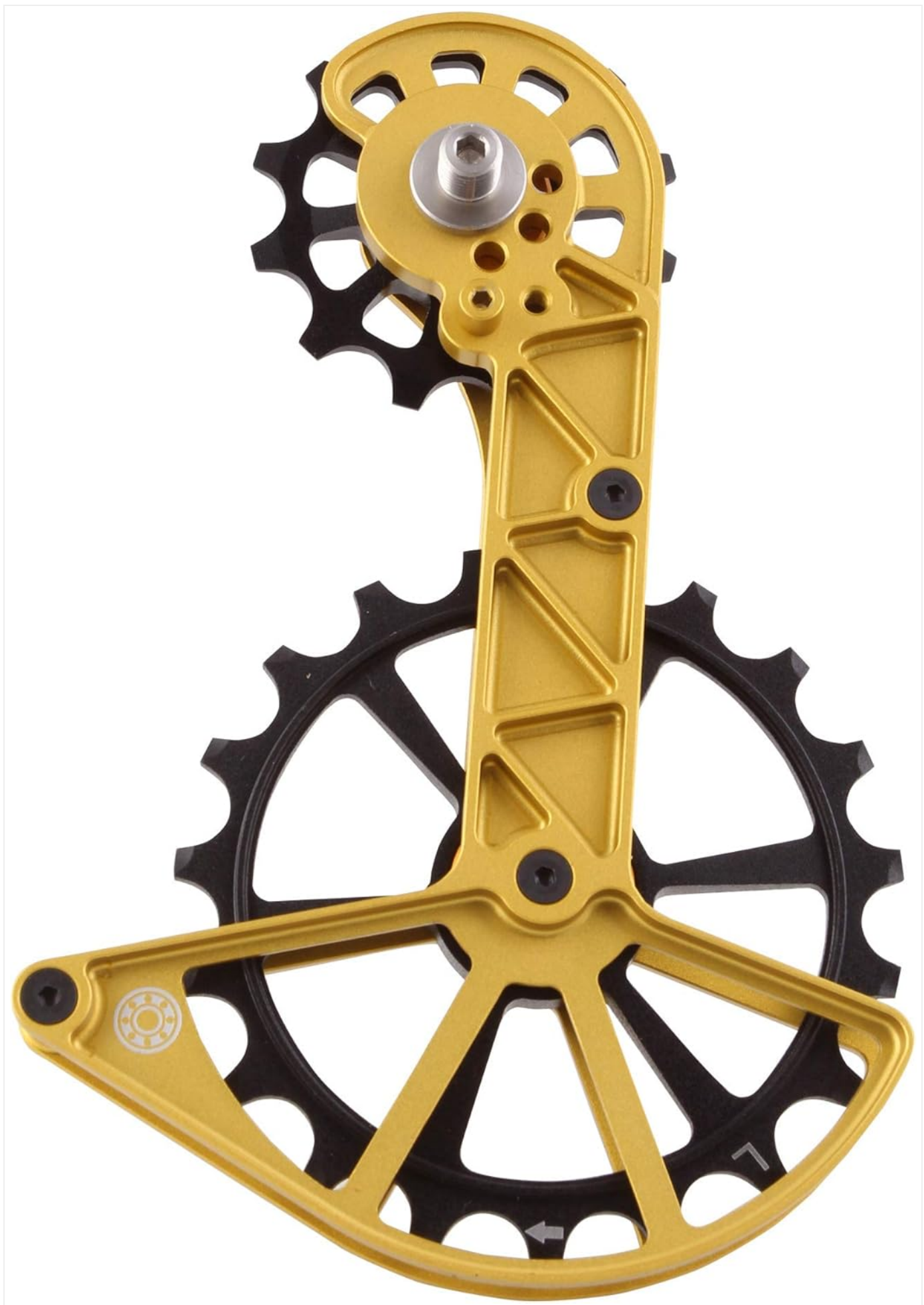
Image: The Kogel Kolossos Oversized Pulley Cage, featuring a gold-anodized aluminum cage and two black oversized derailleur pulleys. The upper pulley is smaller than the lower one, and the cage has a distinctive open design with structural bracing. A bearing symbol is visible on the lower part of the cage, indicating the location of the ceramic bearings.
