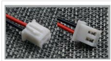
Figure 2: Example of a 2-pin power connector, showing the red (positive) and black (negative) wires.
