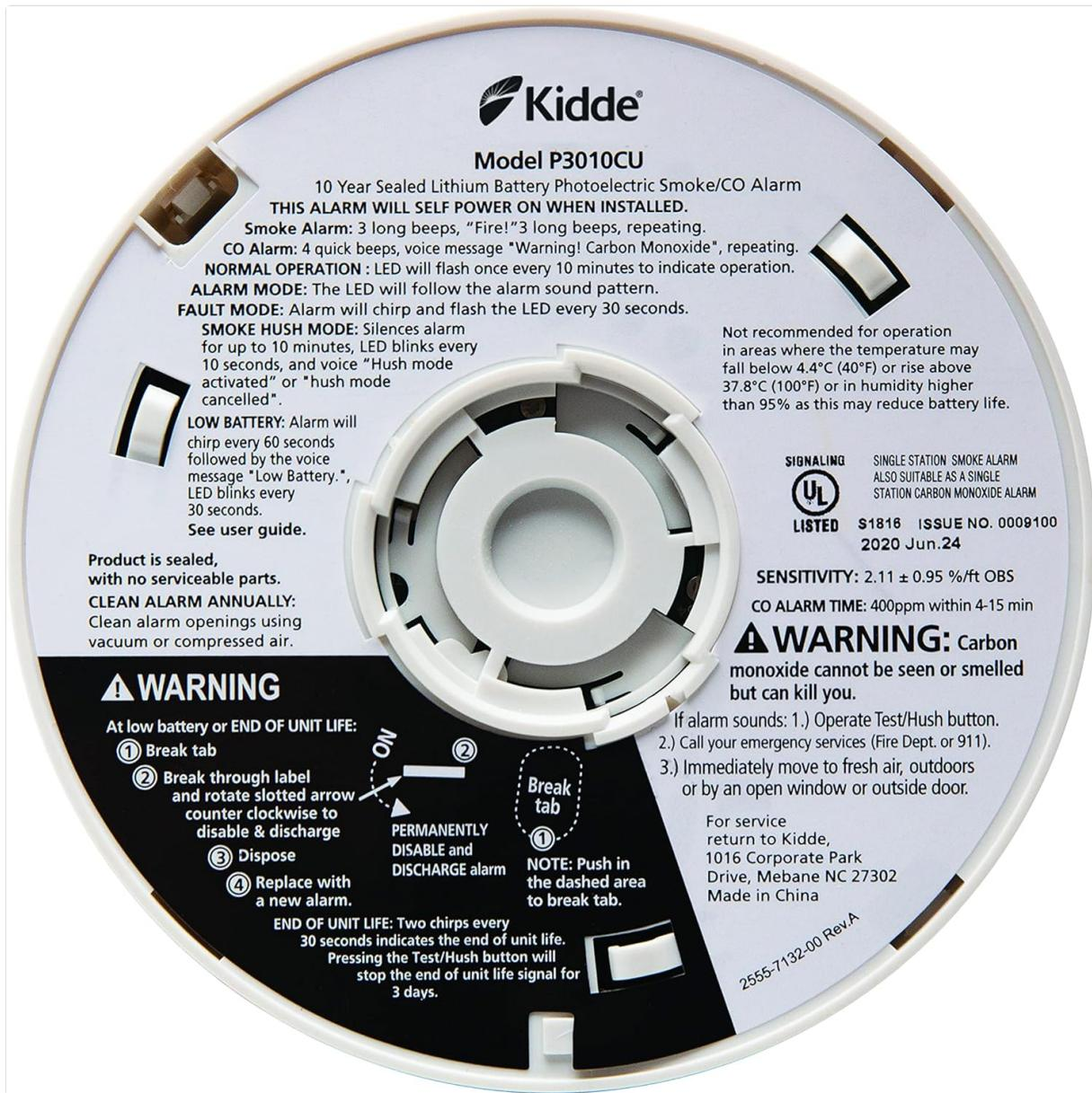
Figure 3: Rear view of the Kidde P3010CU showing the activation mechanism (twist ON/OFF), the permanent disable/discharge tab for end-of-life, and important warnings and instructions.
