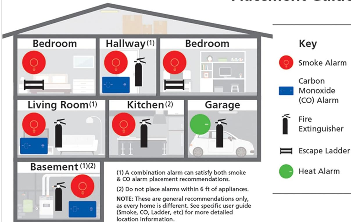
**Figure 2:** Home Safety Product Placement Guide illustrating recommended locations for smoke alarms (red), carbon monoxide alarms (blue), fire extinguishers, and escape ladders within a typical two-story home layout. Combination alarms can satisfy both smoke and CO placement recommendations. Avoid placing alarms within 6 feet of appliances.
