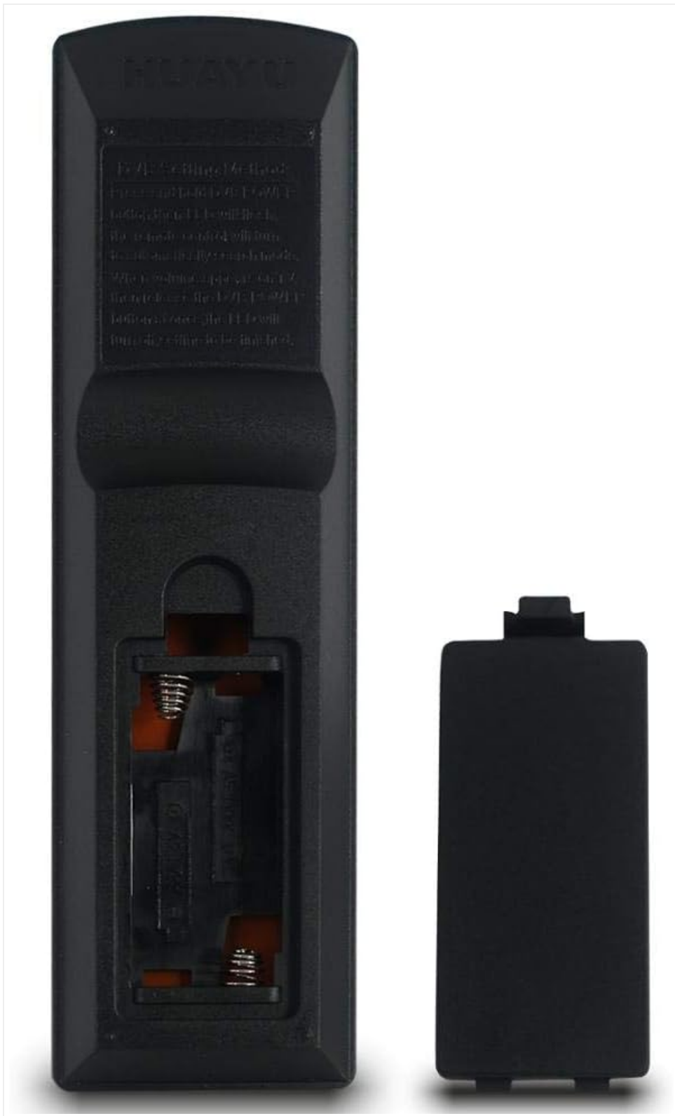
Figure 2.1: Battery compartment with cover removed, showing battery placement.
