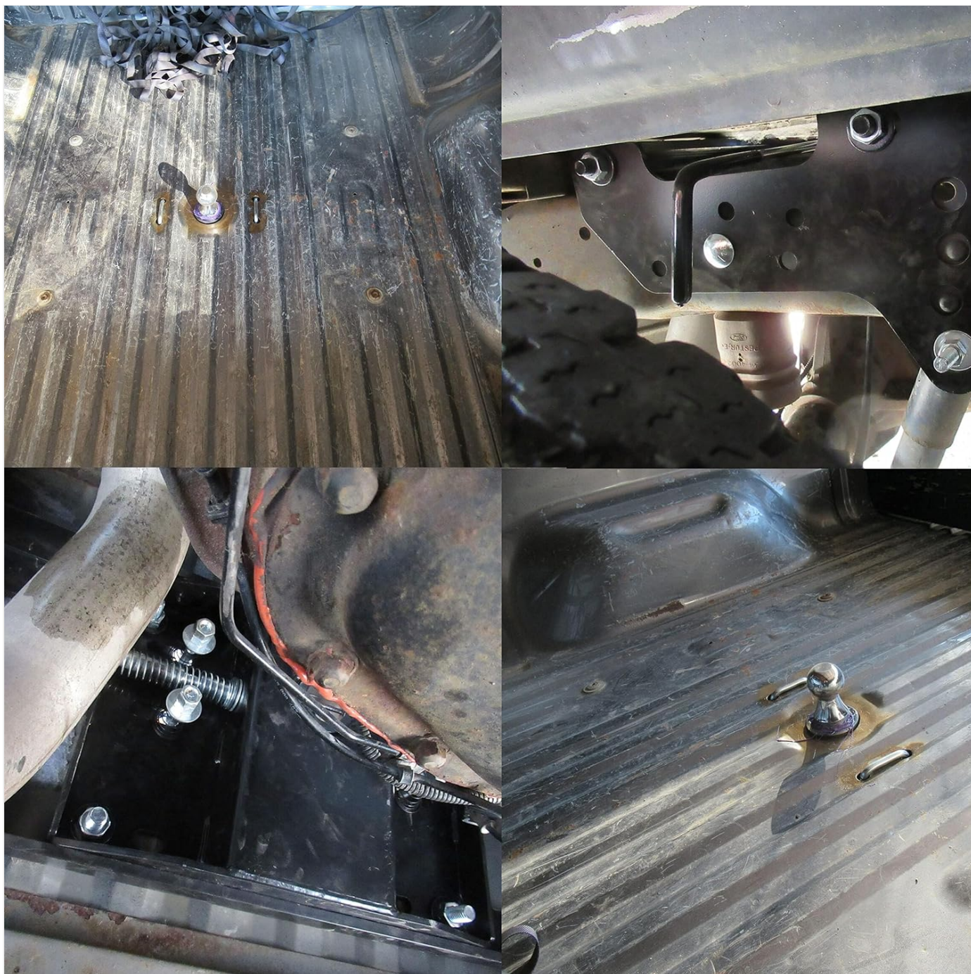
Image 4: Various views of the hitch installed in a truck bed and its undercarriage mounting.
