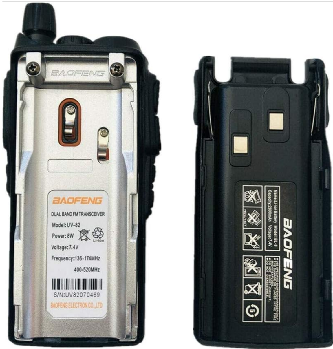
Image: The back of the BAOFENG UV-82 radio with its battery detached, illustrating the battery compartment and the separate battery pack.
