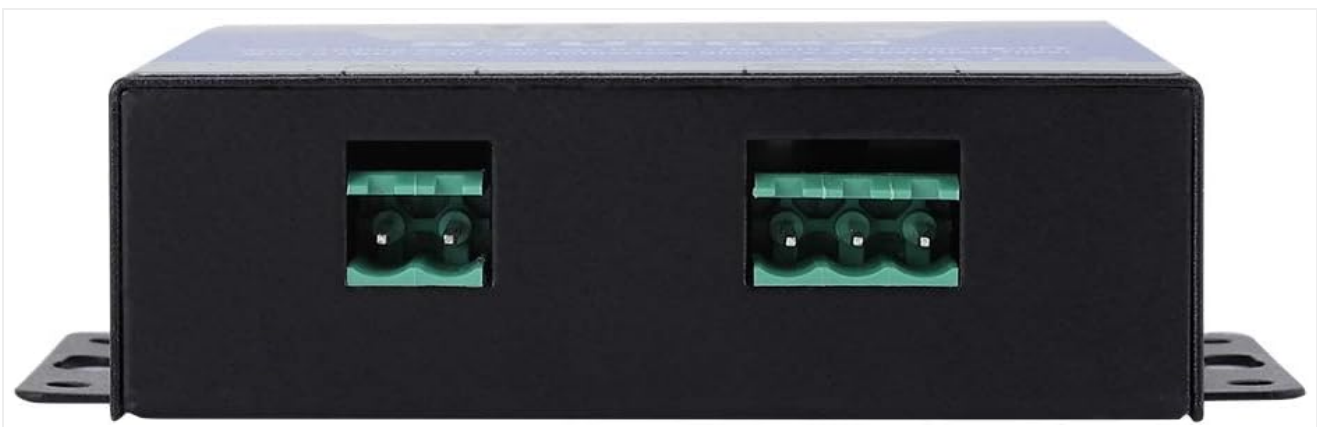
Figure 3: Bottom view of the RTU5024, highlighting the power and relay output terminal blocks.
