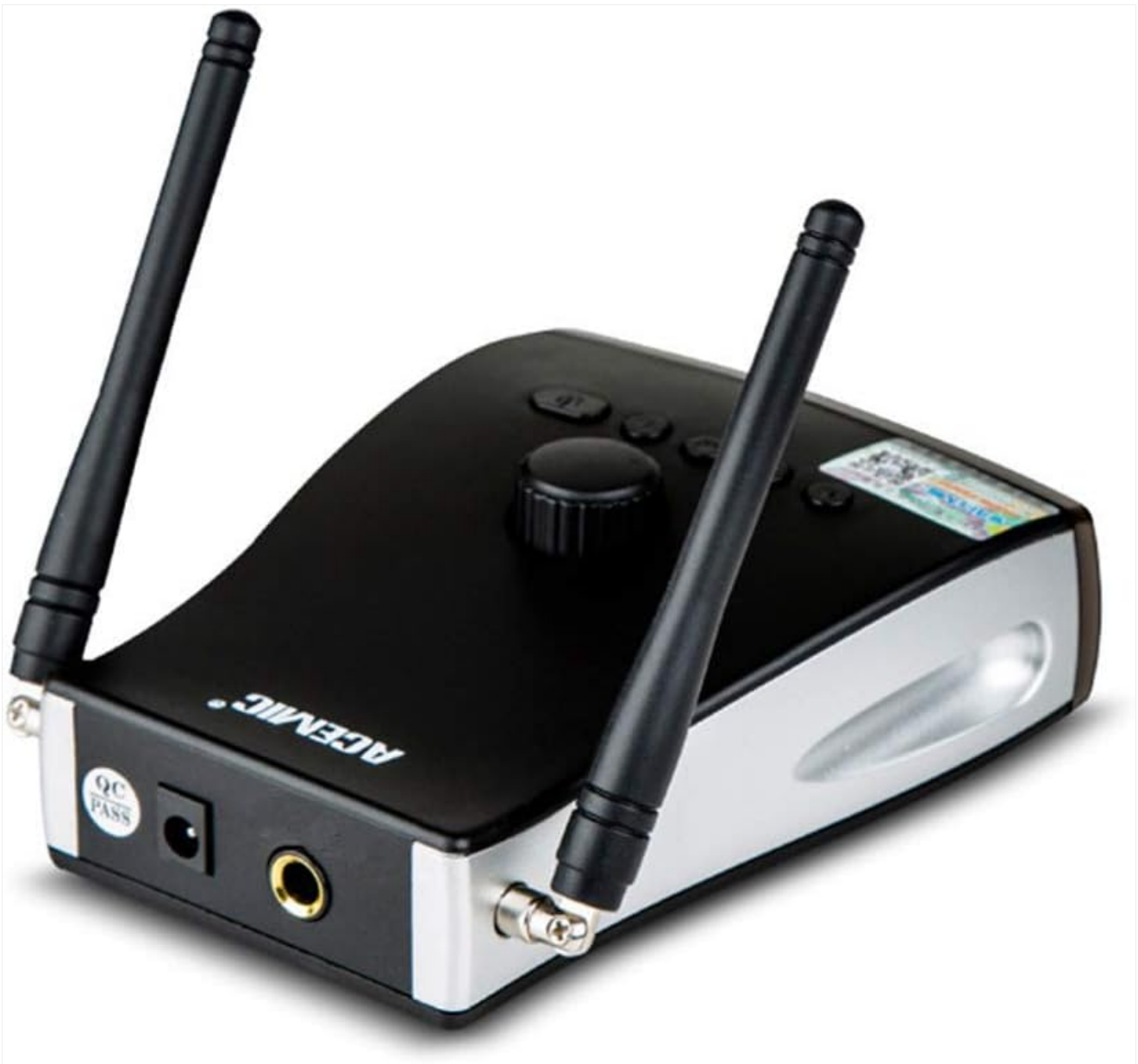
Image: Rear view of the ACEMIC PR/8-ST4 receiver, highlighting the power input and 6.35mm audio output jack, along with the antenna connections.
