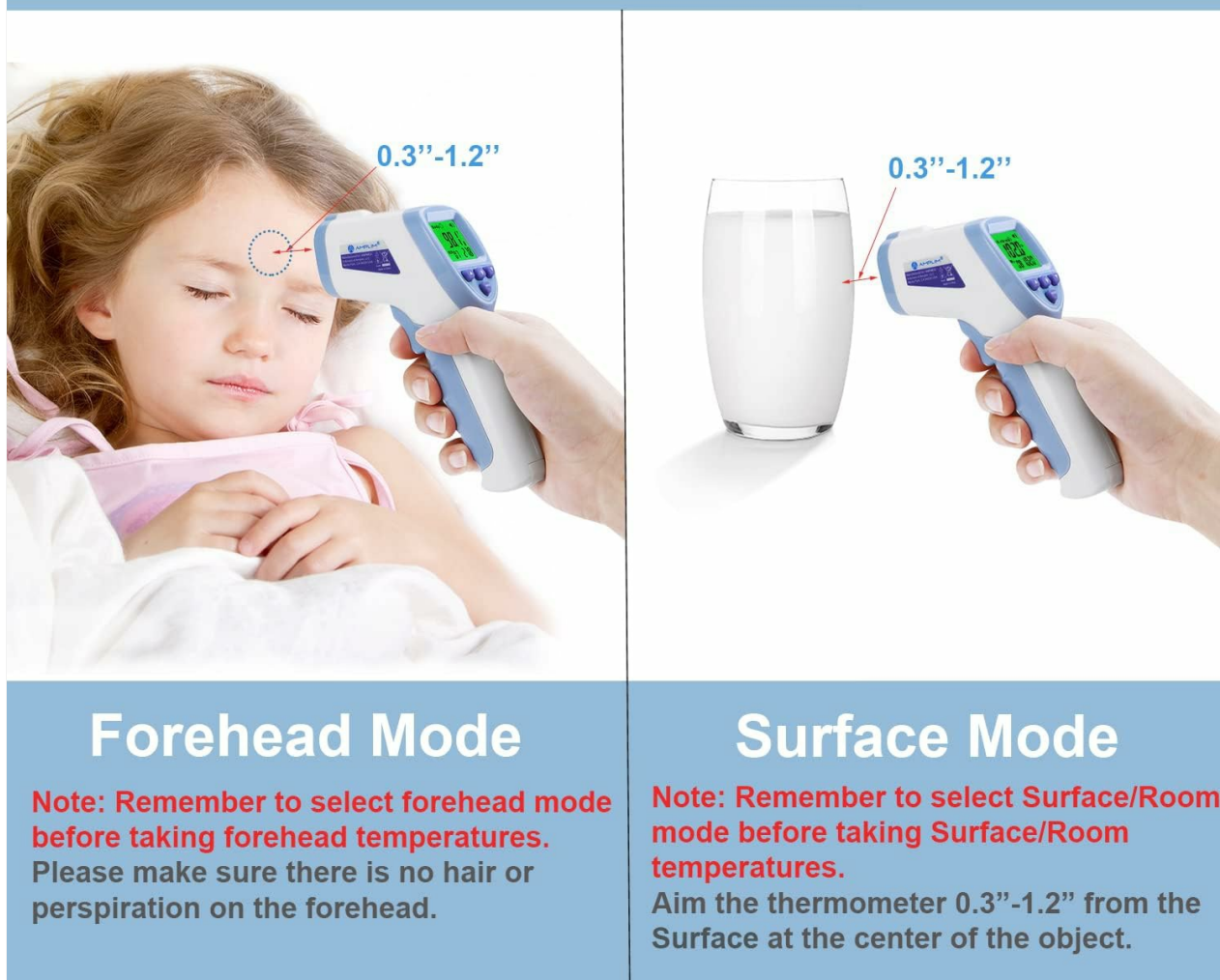
Figure 6: An illustration showing the Amplim thermometer being used in Forehead Mode on a child's forehead and in Surface Mode on a glass of milk, indicating the 0.3"-1.2" measurement distance for both.
