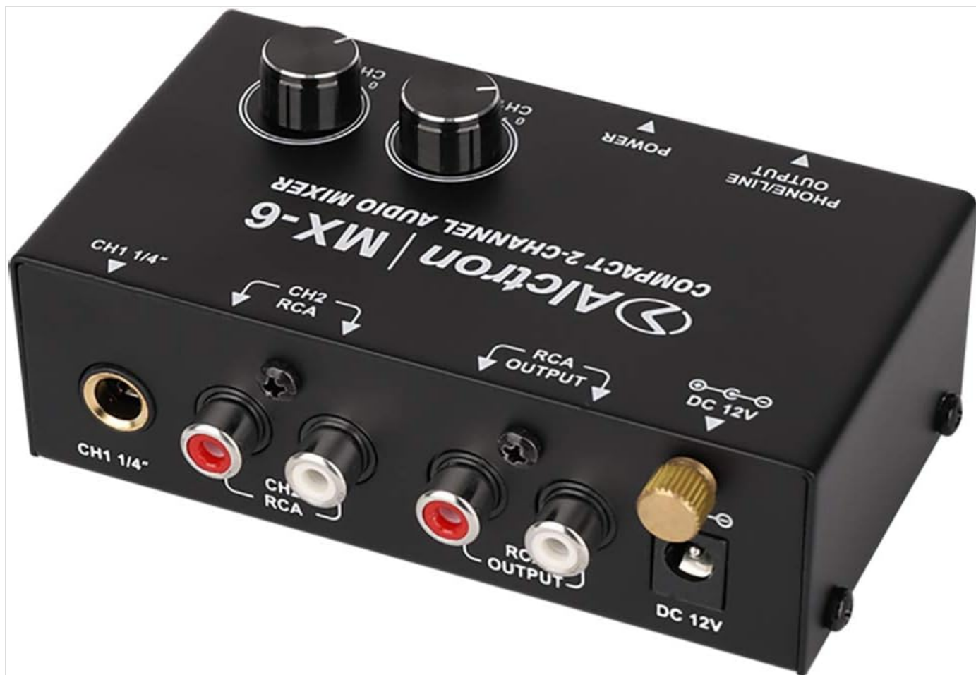
Figure 5.2: Rear Panel View. This image shows the rear panel of the Alctron MX-6. From left to right, it features the CH1 1/4" (TRS) input, CH2 RCA inputs (left and right), RCA OUTPUTs (left and right), and the DC 12V power input jack.
