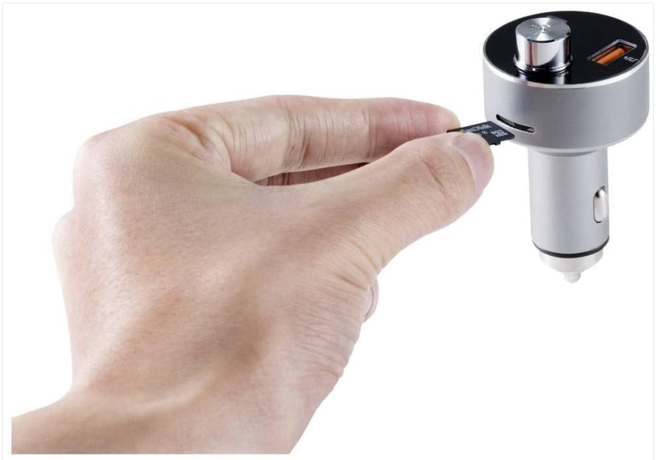
Figure 4: A hand demonstrating the insertion of a Micro SD card into the dedicated slot on the side of the FM Transmitter for direct audio playback.
