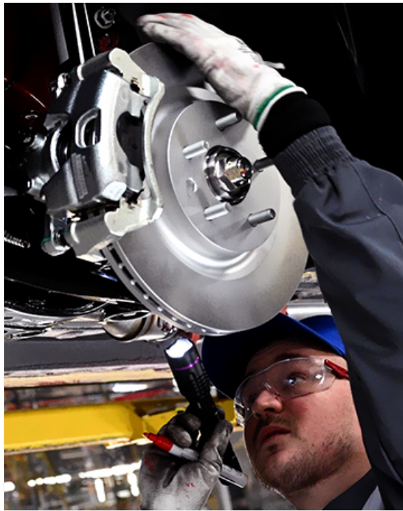
Figure 5: Securing the brake caliper after pad installation.
