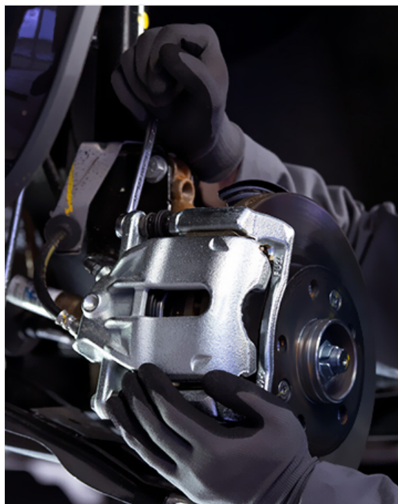
Figure 4: Proper installation of a brake pad into the caliper bracket.
