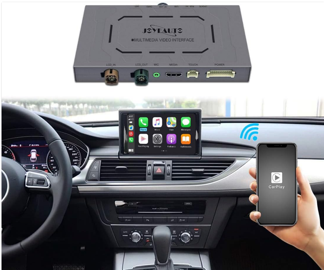
Image 1.1: The JOYEAUTO retrofit module and its integration with an Audi vehicle's display, showing CarPlay in action.
