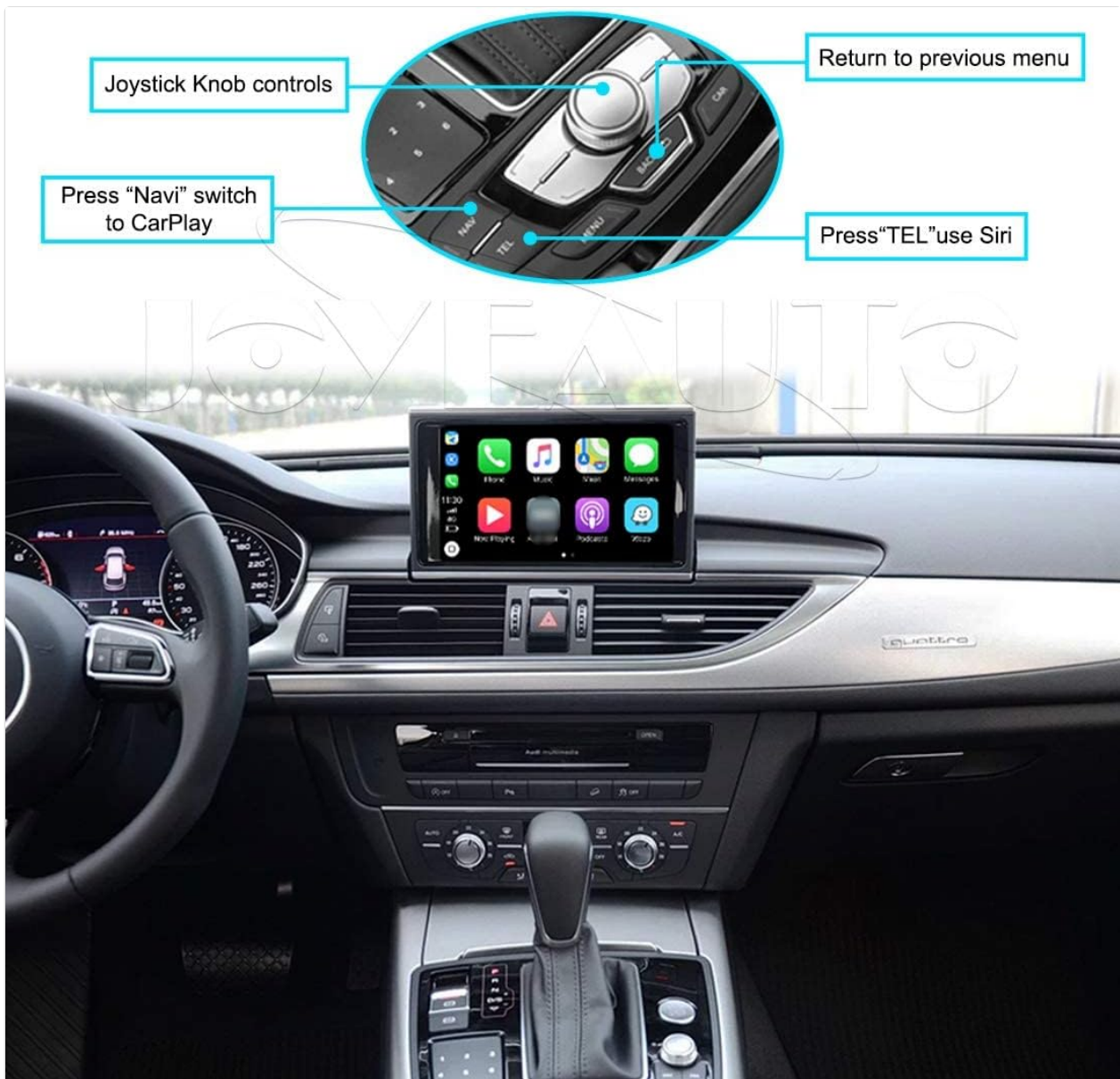
Image 3.4: Highlights the use of the original Audi joystick knob for controlling the CarPlay interface, with labels for "Press 'Navi' switch to CarPlay" and "Press 'TEL' use Siri".
