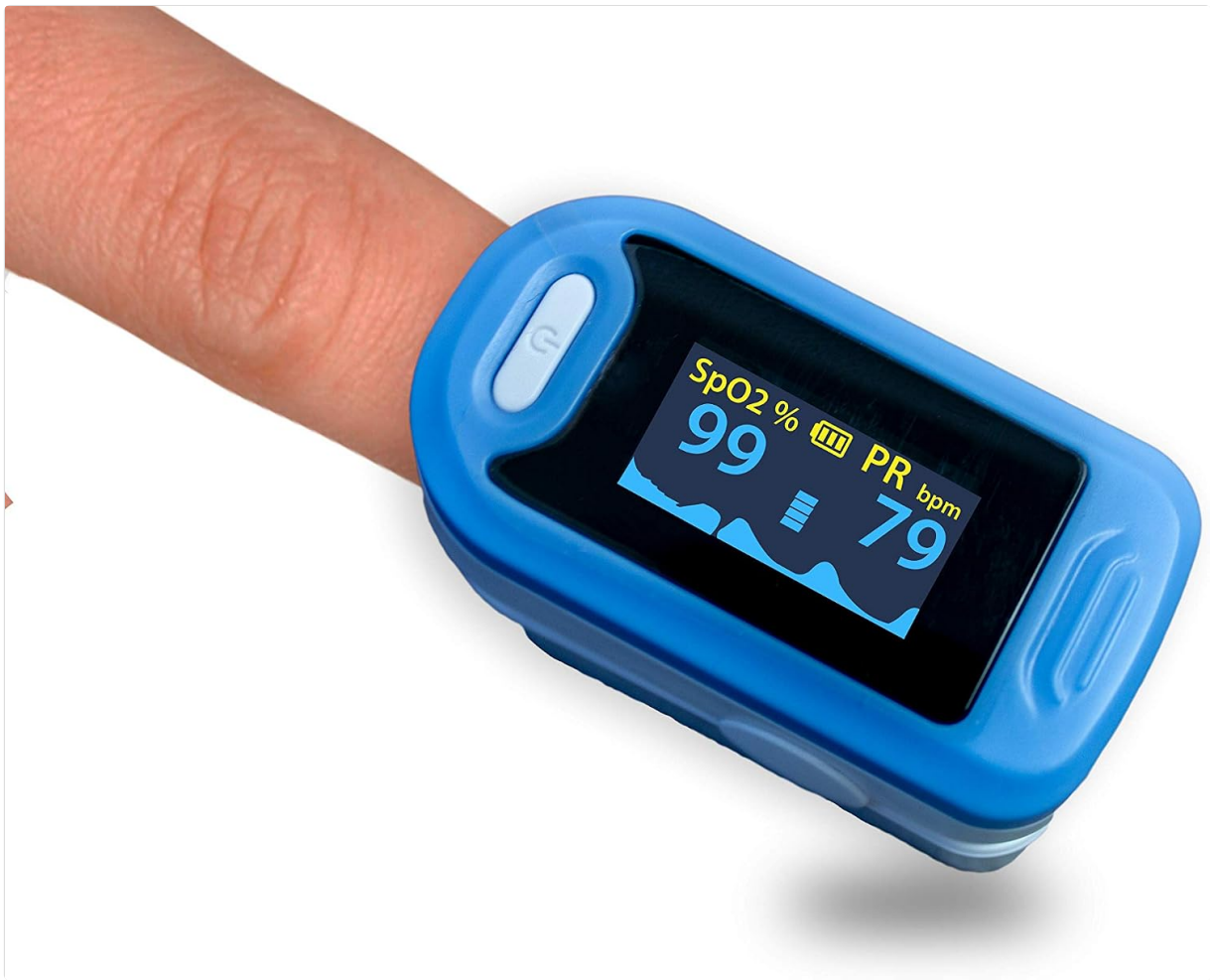
Figure 4: Proper placement of the finger in the oximeter for measurement.
