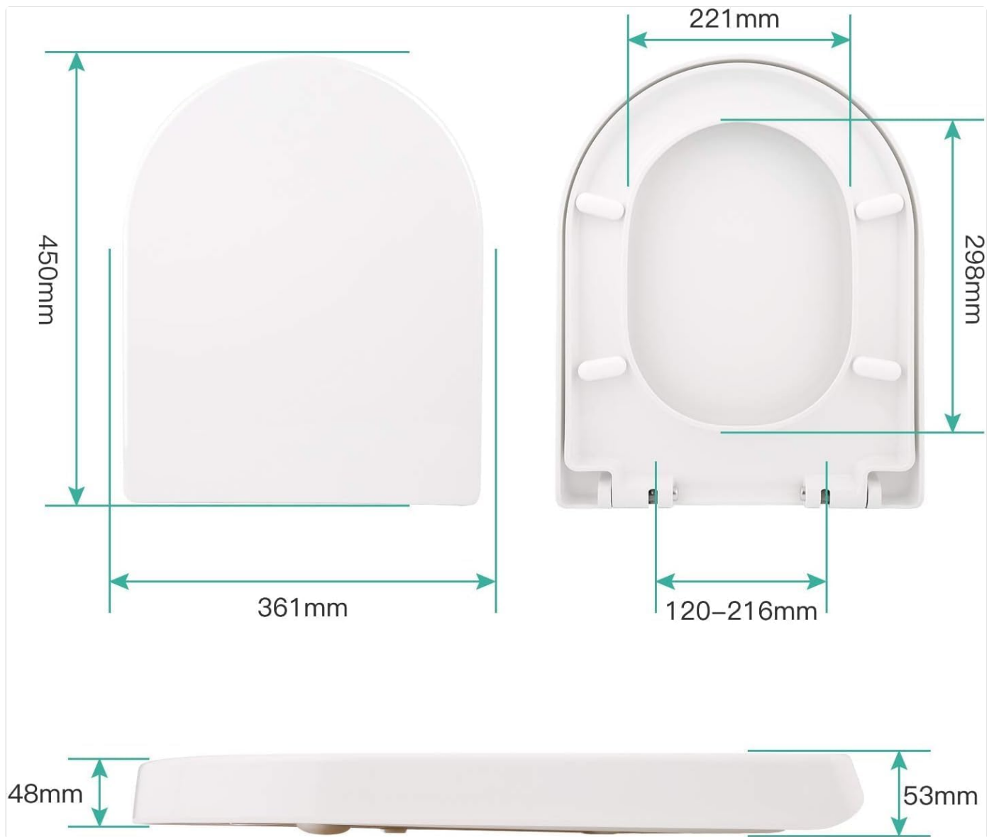
Image: Detailed diagram illustrating the dimensions of the Himimi Universal Toilet Seat, including length, width, and hinge spacing.
