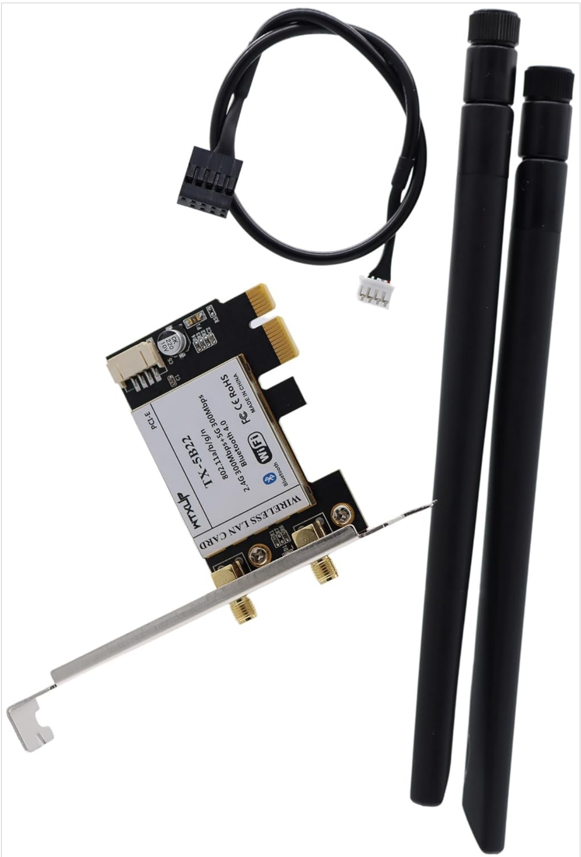
Image 3: The AR5B22 WLAN card with the low profile bracket, demonstrating its adaptability for different PC case sizes.
