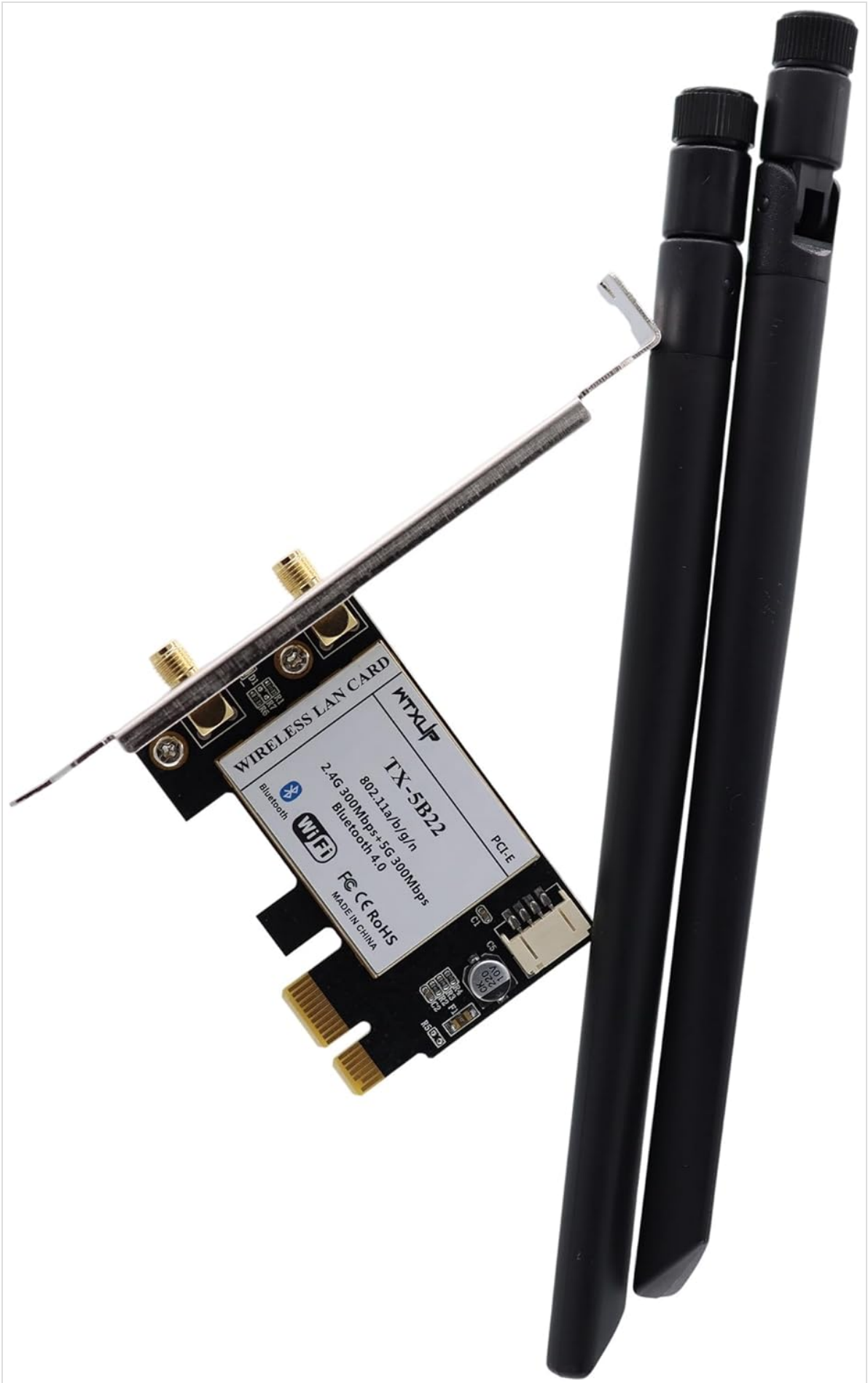
Image 4: The fully assembled AR5B22 WLAN card with antennas and low profile bracket, ready for use.
