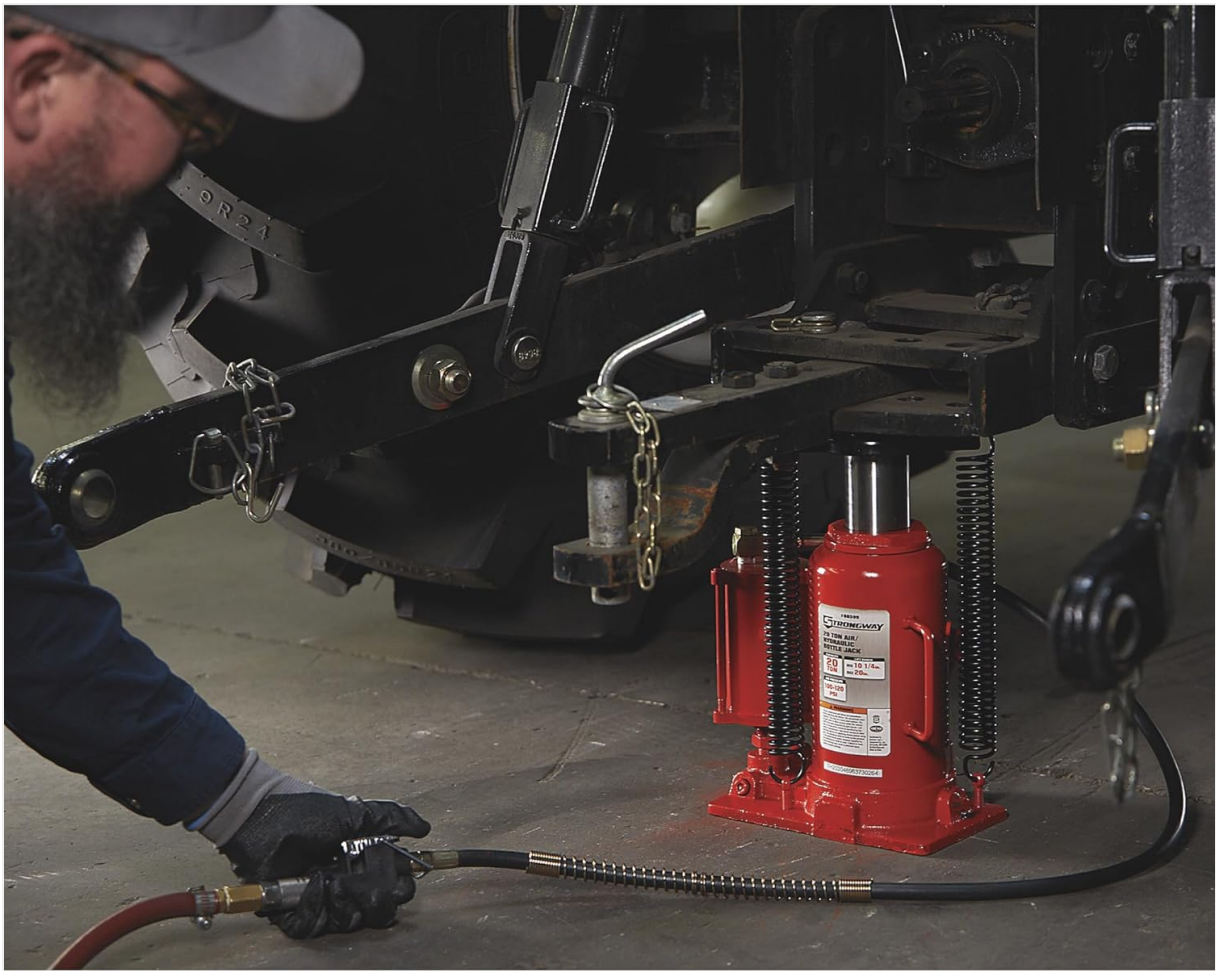
Figure 5: The jack in operation using an air hose, lifting a heavy load. This illustrates the air-powered lifting mechanism.
