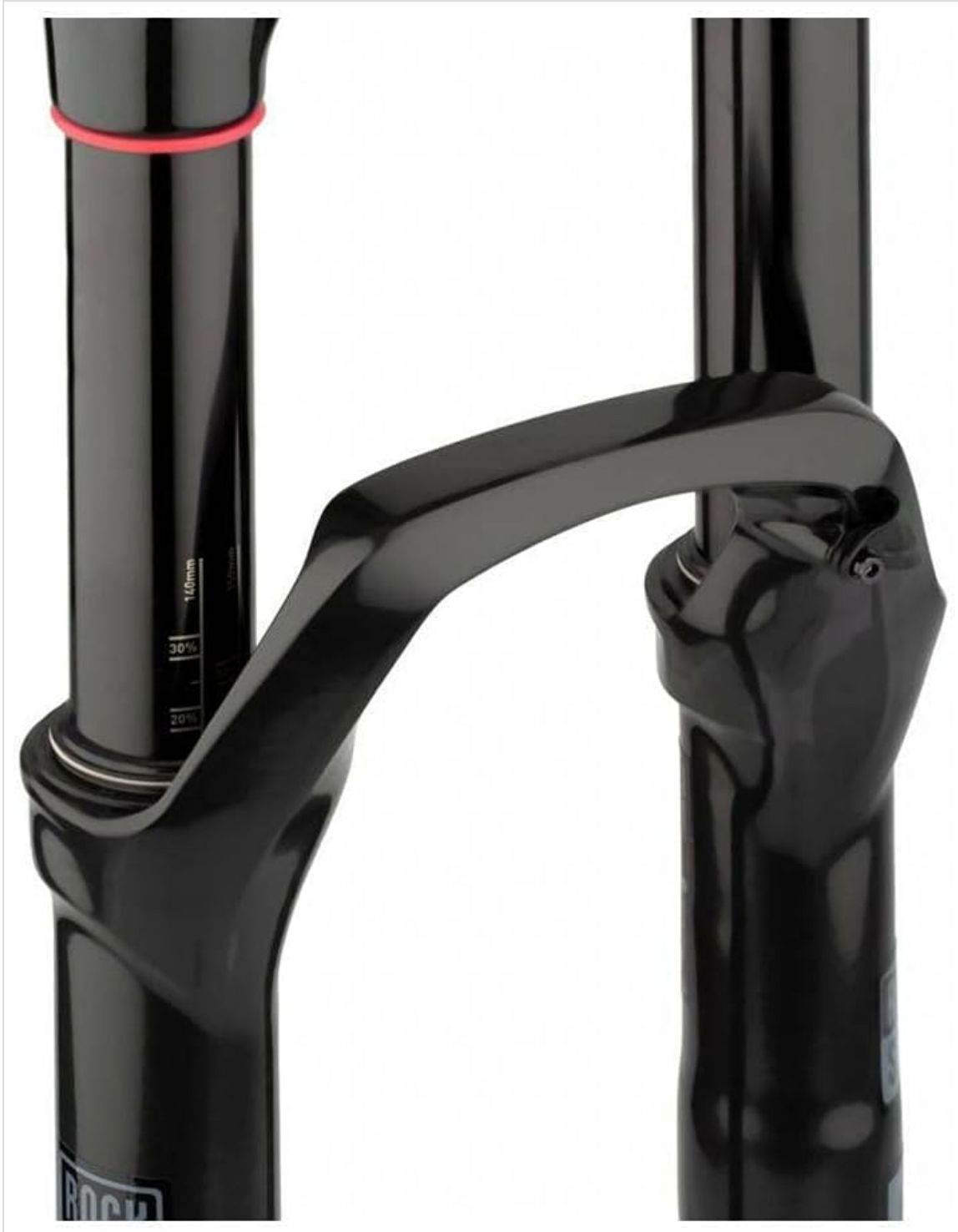
Figure 2.2: The fork stanchion displaying sag indicators, which aid in setting the correct suspension sag.
