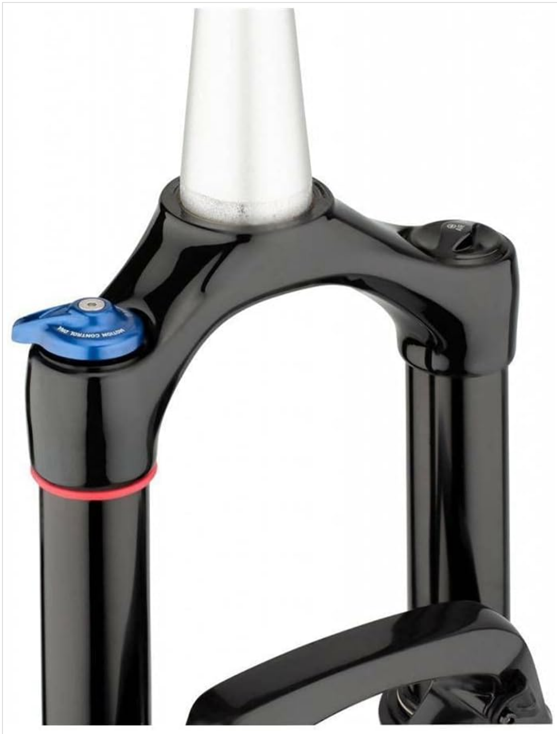
Figure 2.1: Top of the left fork leg showing the blue adjustment knob and the location for air pressure adjustment.
