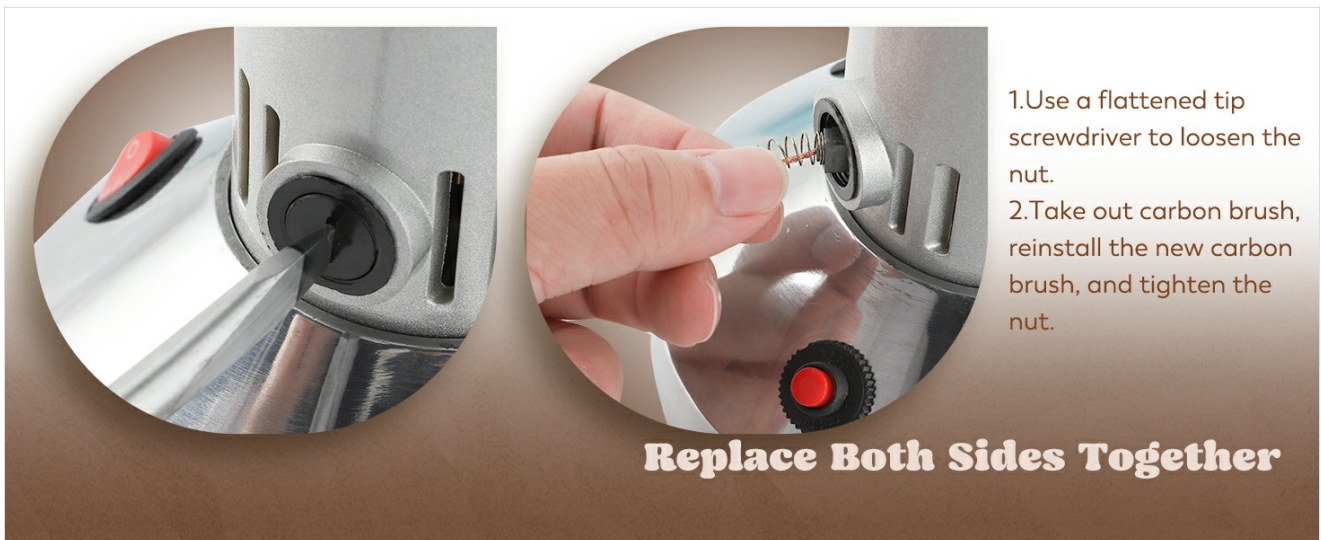
Image: A visual guide demonstrating how to replace the carbon brushes. It shows using a screwdriver to access and replace the brushes, advising to replace both sides simultaneously.
