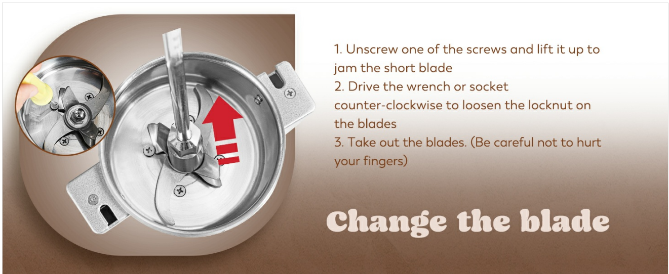
Image: A step-by-step visual guide on how to replace the grinding blades. It shows how to unscrew, loosen the locknut, and remove the blades, emphasizing careful handling.
