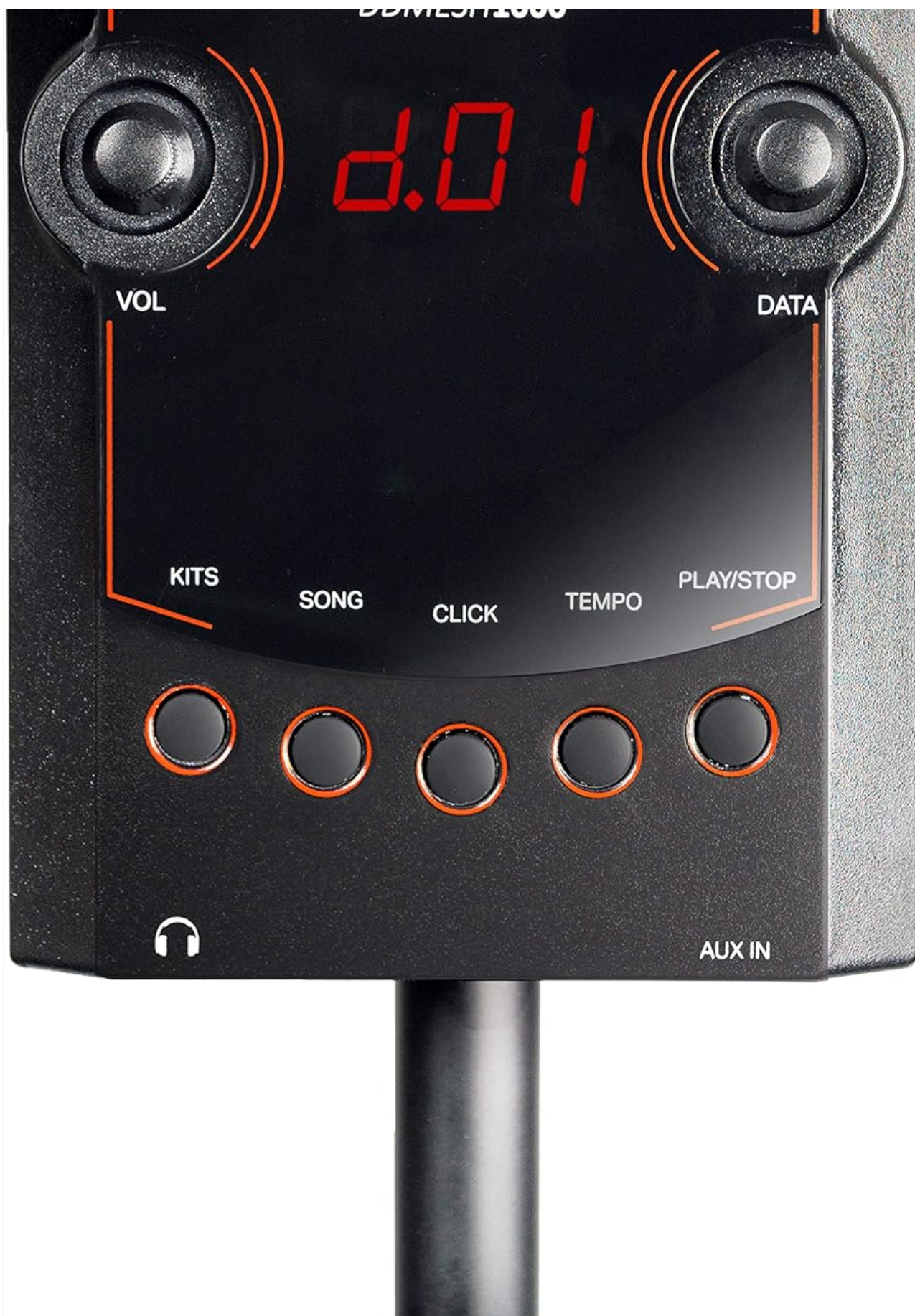
Image: Front panel of the drum module, showing the digital display, VOL and DATA knobs, and buttons for KITS, SONG, CLICK, TEMPO, and PLAY/STOP, along with headphone and AUX IN jacks.
