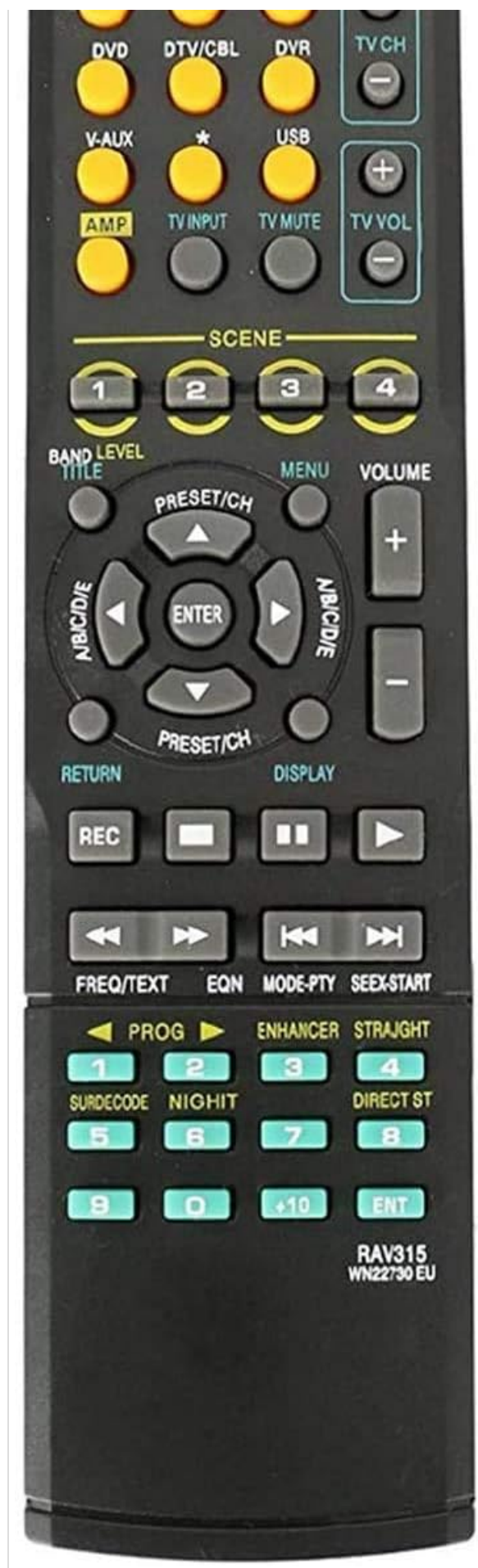
Image Description: A full front view of the Elek pia RAV315 replacement remote control. The remote is black with various buttons in different colors (red, yellow, green, gray) clearly labeled for functions such as power, input selection, volume, channel, menu navigation, and playback controls. The model number "RAV315 WN22730 EU" is visible at the bottom right.
