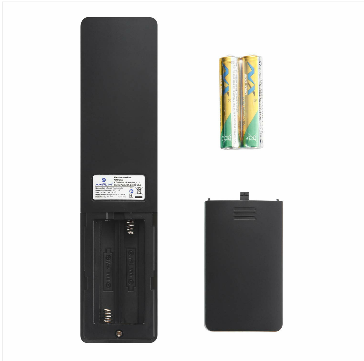
Figure 2: Included Components and Battery Installation
