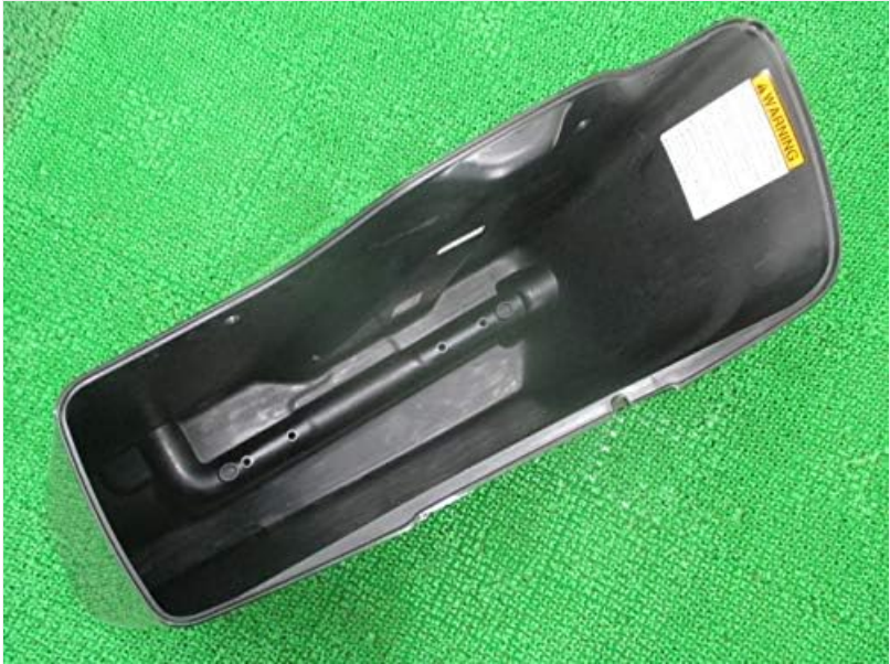
Figure 3: Interior view of the pannier case, illustrating the internal structure and mounting points for attachment to the motorcycle.
