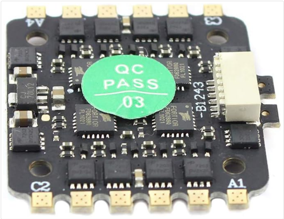
Figure 6: Detailed bottom view of the HAKRC ESC, revealing the main chip and connector.
