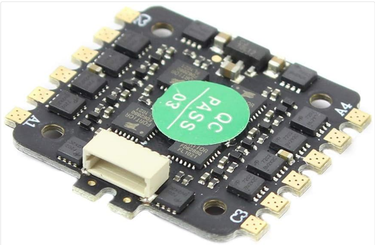
Figure 5: Bottom view of the HAKRC ESC, showing the 'QC PASS' sticker and main connector.
