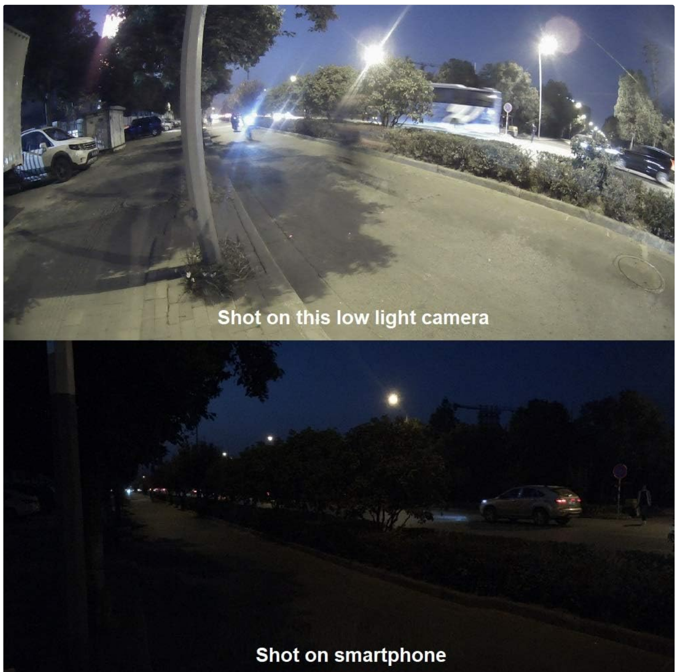
Figure 3: Demonstrates the superior low-light performance of the Arducam camera compared to a standard smartphone camera.
