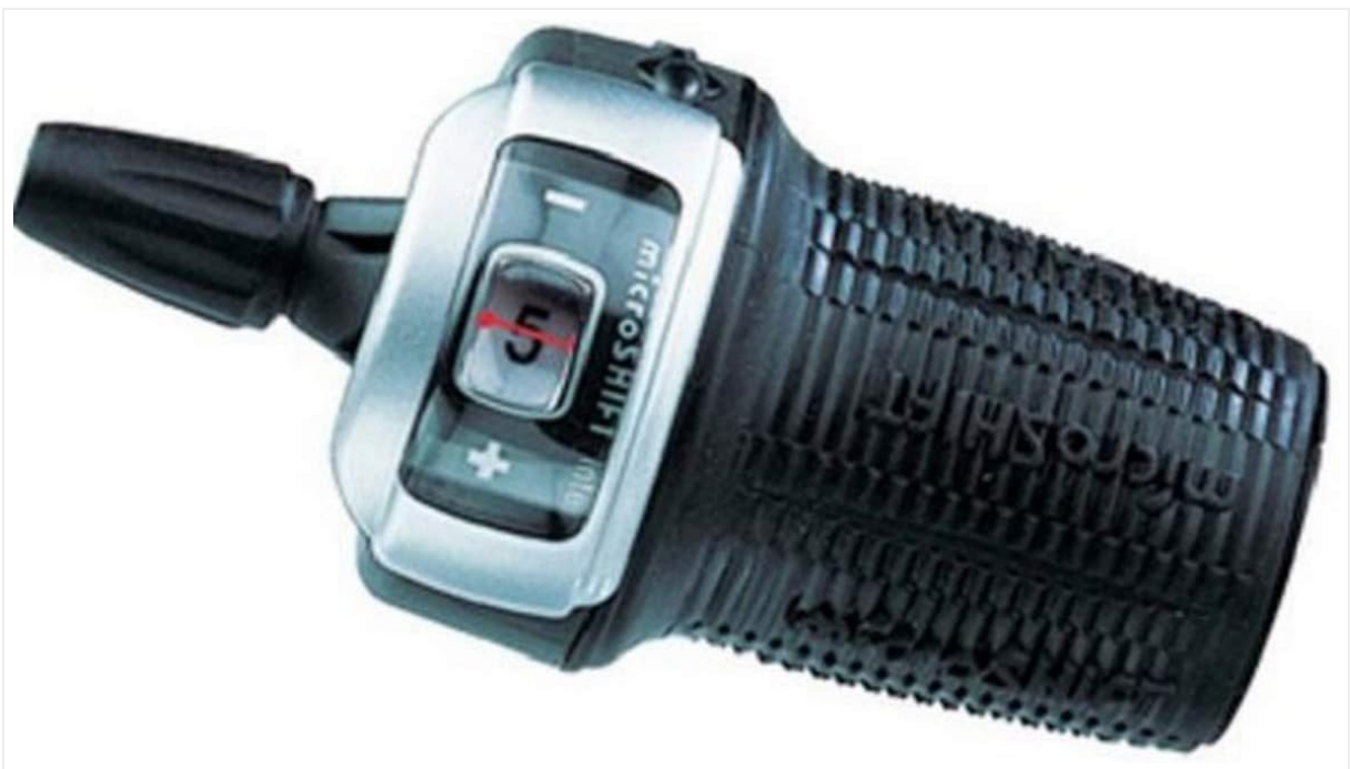
Image 1.1: The microSHIFT DS85 Right Twist Shifter, showing its ergonomic design and optical gear indicator.
